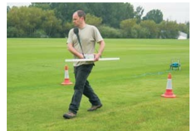
GEM-2 Multi-frequency Exploration depth up to 10m
