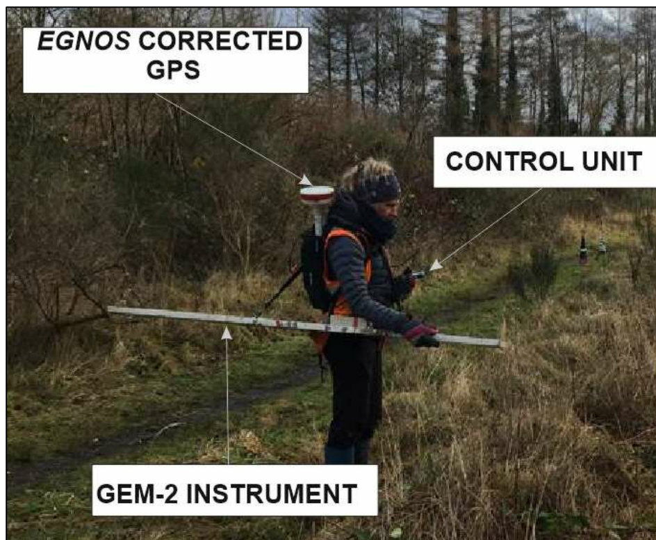
Plate 4: Electromagnetic survey set-up on site in Zone 4.
