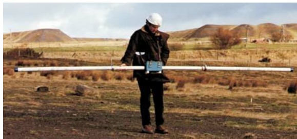
EM-31 Single frequency Exploration depth ~3 to 5m
