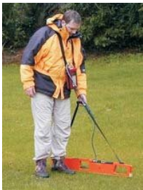
EM-38 Single frequency Exploration depth ~1.5m
