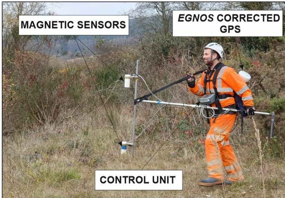
Plate 3: Magnetic survey set up on site in Zone 4.
