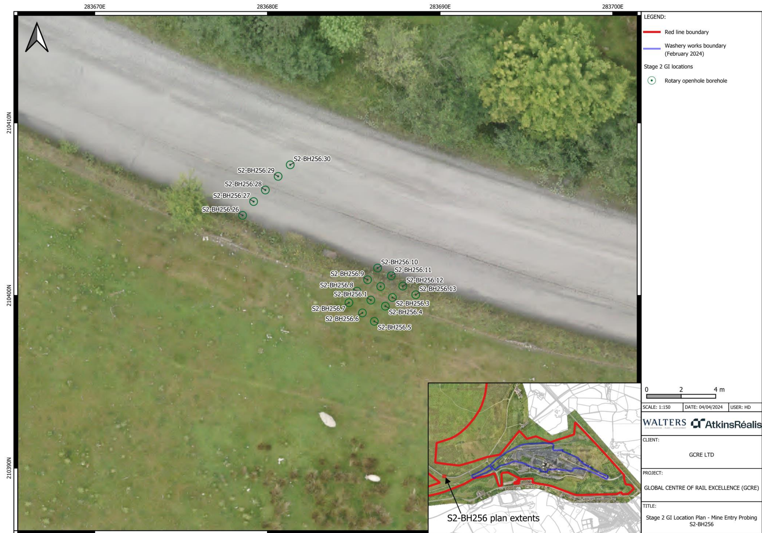
Figure 3-7: Stage 2 GI Location Plan – Mine Entry Probing S2-BH256 (Imagery copyright AtkinsRéalis)
