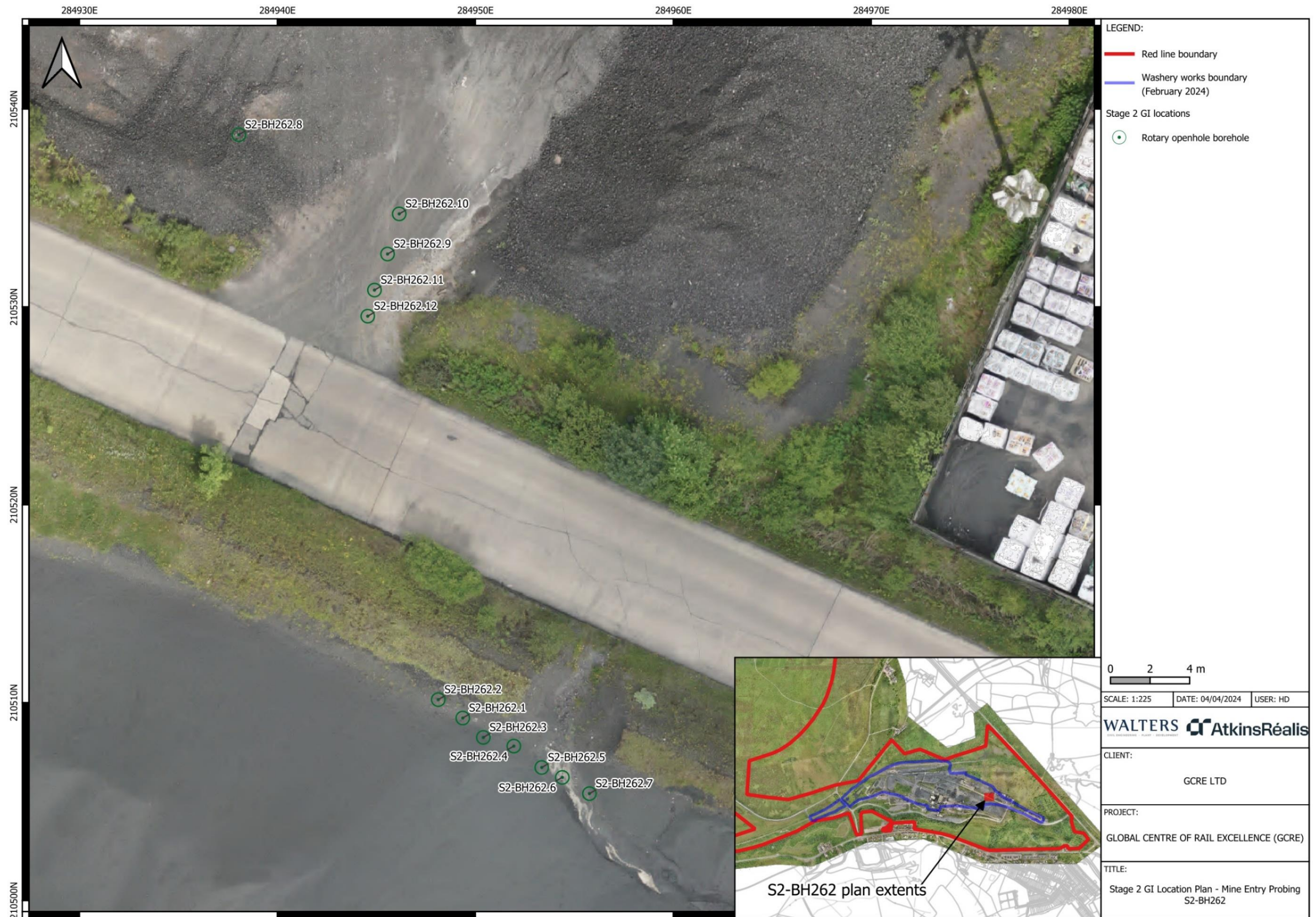
Figure 3-11: Stage 2 GI Location Plan – Mine Entry Probing S2-BH262 (Imagery copyright AtkinsRéalis)
