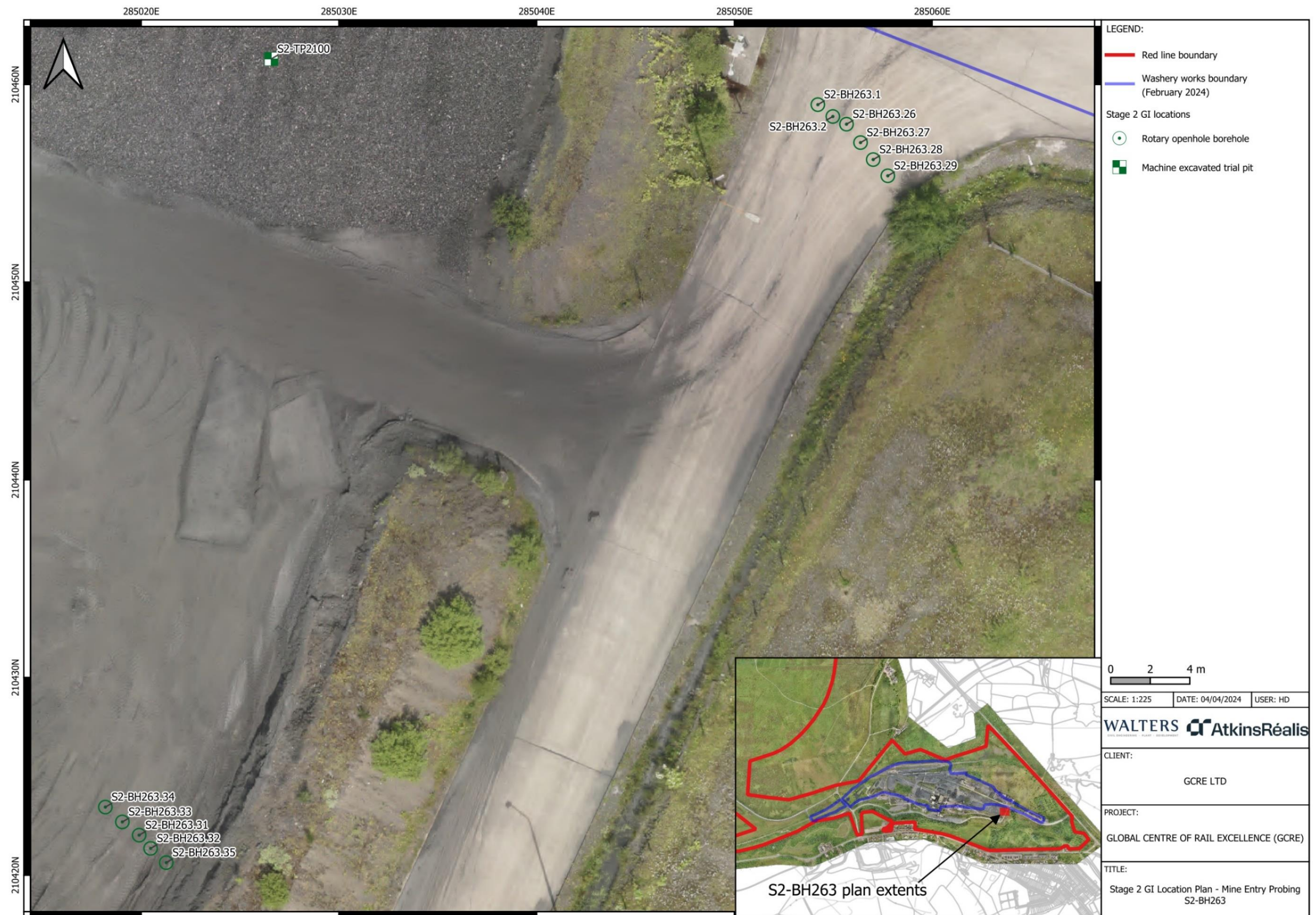
Figure 3-12: Stage 2 GI Location Plan – Mine Entry Probing S2-BH263 (Imagery copyright AtkinsRéalis)
