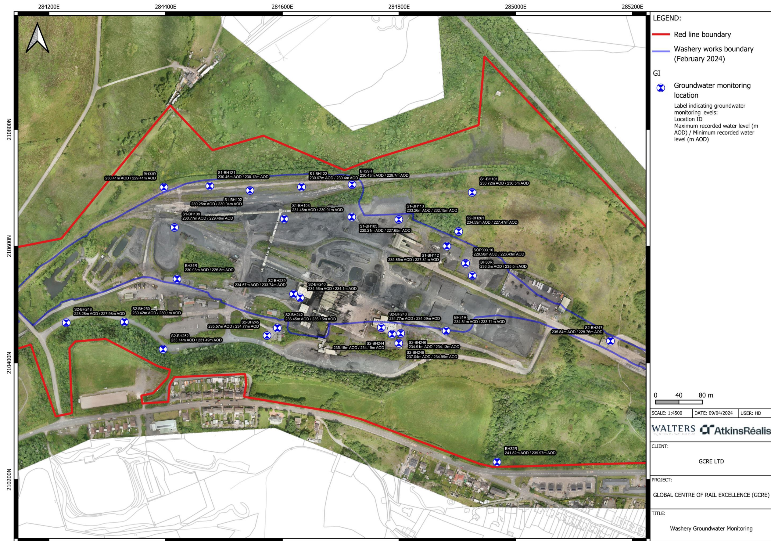
Figure 4-8: Washery Groundwater Monitoring (Imagery copyright AtkinsRéalis)
