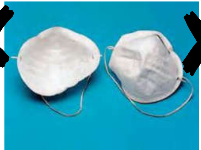
Figure 61 Wrong type of RPE which has been screwed up in a pocket
