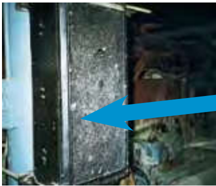
Figure 37 Asbestos debris on an electrical box, adjacent to a machine which was used to make bituminous roofing felt containing asbestos
