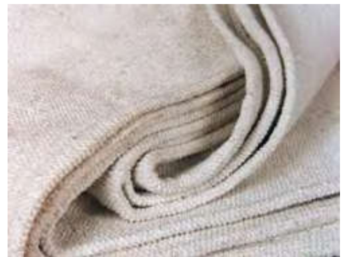
Figure 9 Asbestos fire blanket
