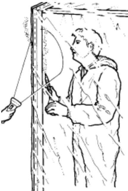
Figure 54 Testing seal with a smoke tube, with second person using a torch to check for smoke leaking from seals
