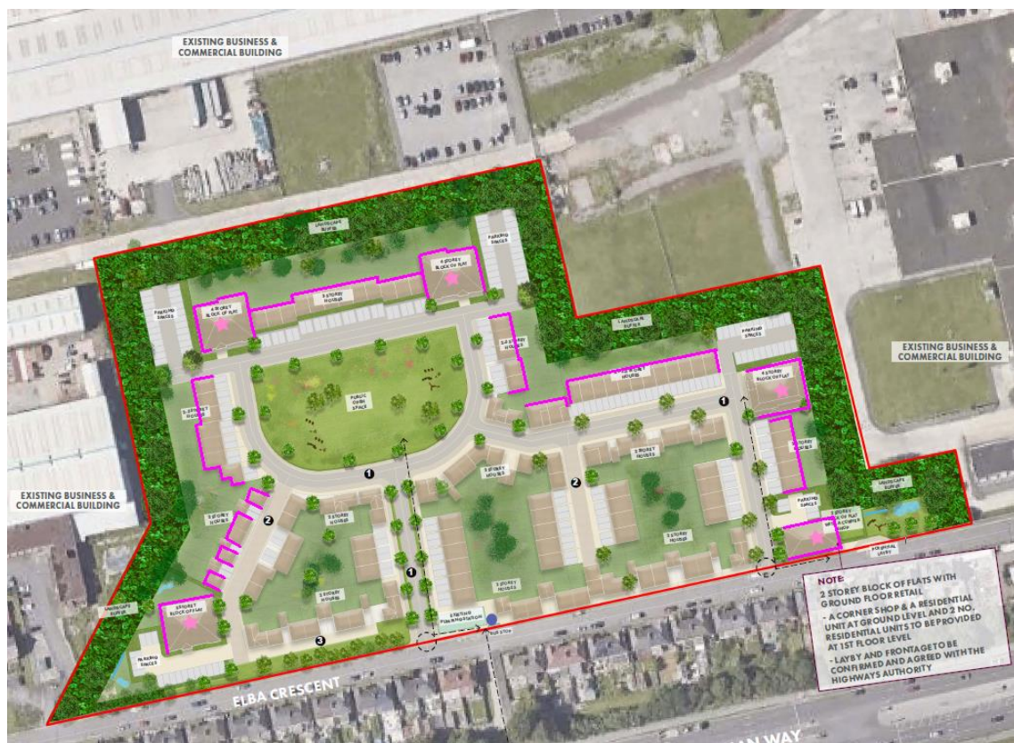
Figure 6.1 – Façades Requiring Additional Sound Insulation Measures
