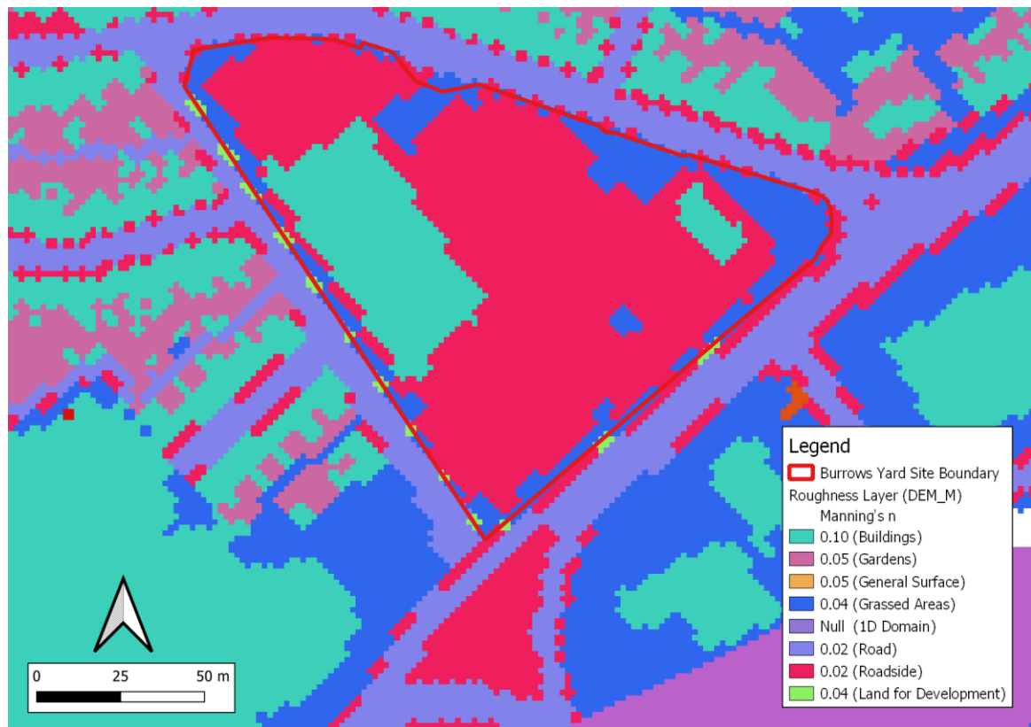
Figure 3-2: Post-development site roughness
