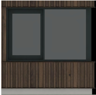
3 Pvc thermally broken aluminium windows frame - colour: ral 9011
