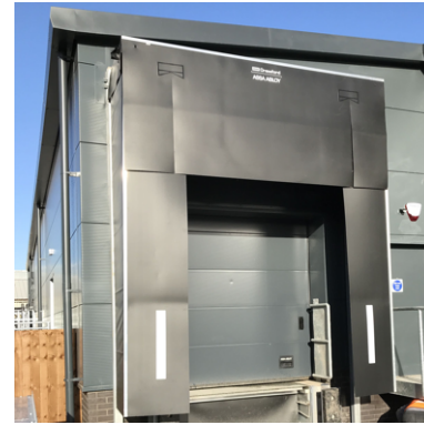
9 Sectional overhead loading bay door - pvf coated steel, ral 7016 (anthracite). Curtain Dock Shelter, colour black
