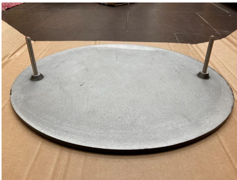
Figure 2 Fittings screwed into studs on back face of plaque
