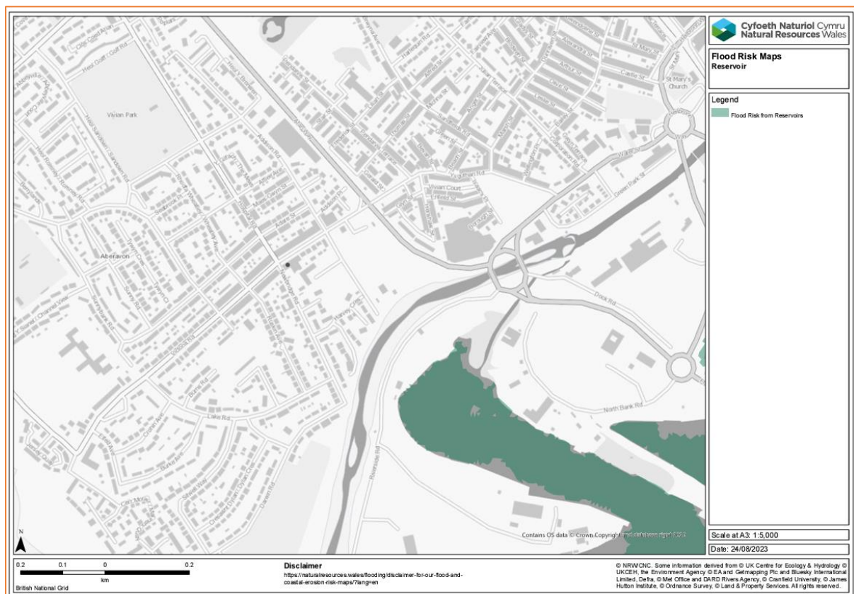
Figure 13: Extract from Natural Resources Wales risk of flooding from reservoirs (Source: NRW)
