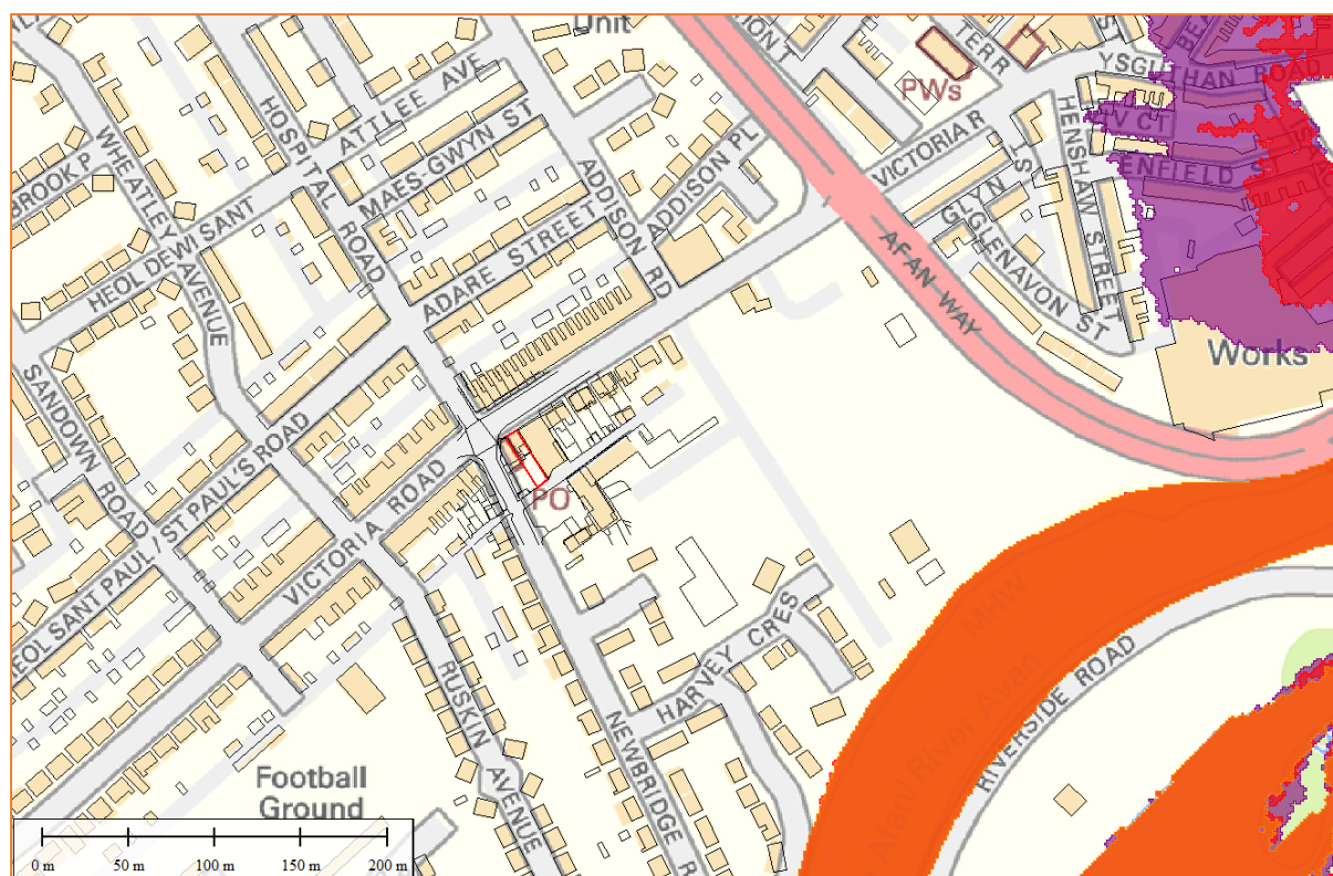
Figure 11: Modelled 1:100 year (orange), 1:100 year + CC (red) and 1:1000 year (purple) fluvial flood extents (Source: NRW, OS Mapping)
