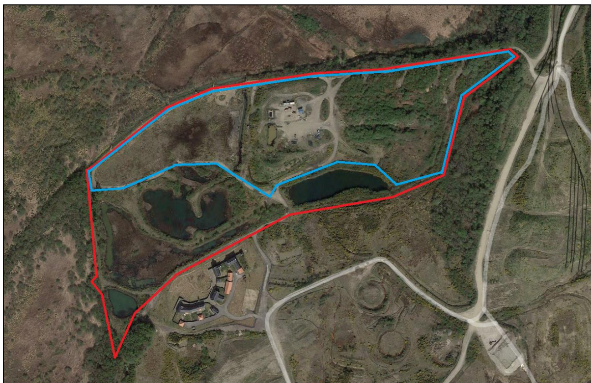
Figure 1: Original permit area (in red), and the site under consideration in this assessment (in blue). Area inside red line, but outside blue line has been subject to a partial surrender in 2013.
