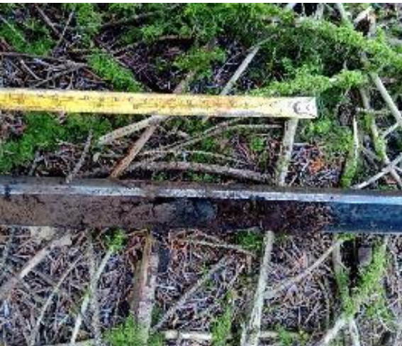
Photograph 10.10: Core from the centre of T3 demonstrating dry soil with high organic content ~0.1 m depth on top of clay.
