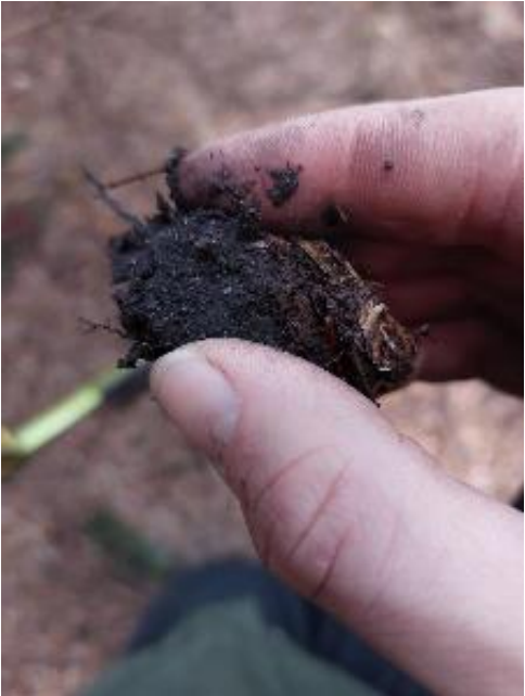
Photograph 10.11: Taken at location of T17 soil shows evidence of sand and grains.
