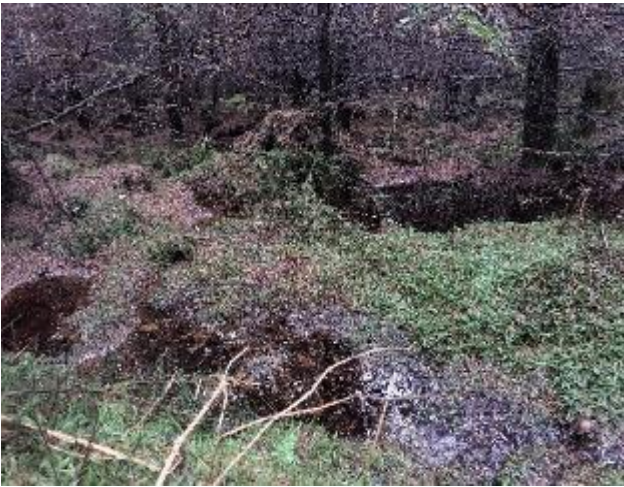
Photograph 10.9: T18, pooling water directly on top of clay. Ridges in area developed with soils from furrows.
