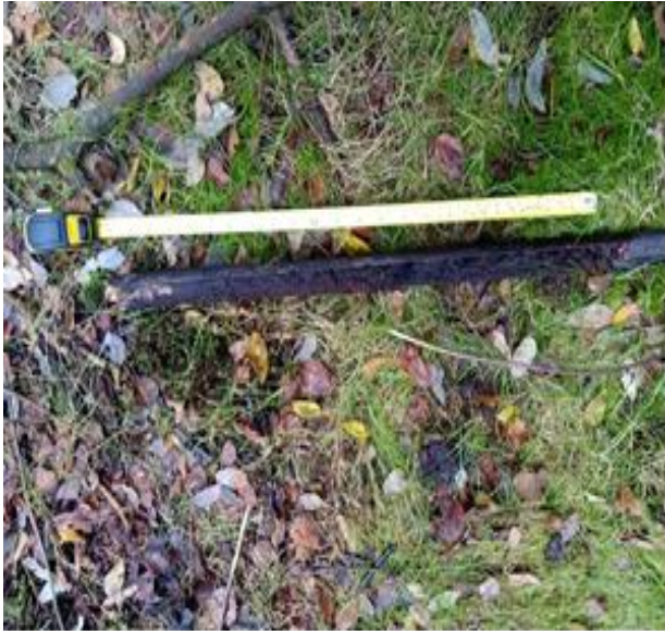
Photograph 10.12: Core at design chill T7 shows some peat, but core was in a small deciduous part of the area. 0.45 m peat, low water content.
