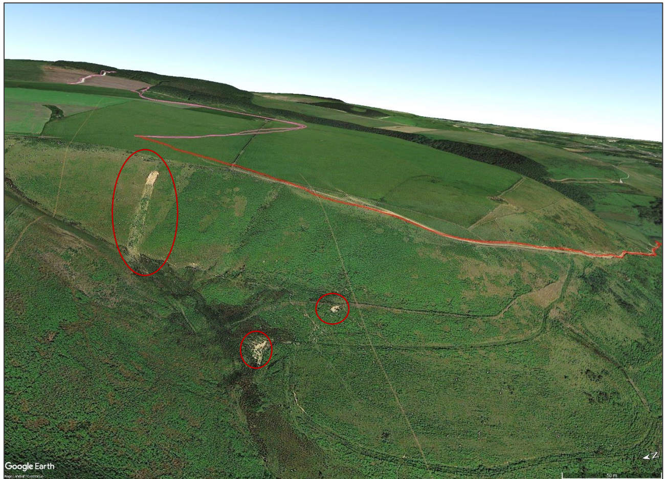
E1: Google Earth Satellite Imagery (2013) with relic landslides circled in red. Image is facing the west side of the existing farm track on the eastern side of the Cwm y Geifr valley.
