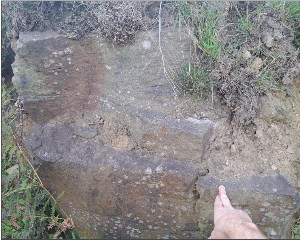
Figure A2: Sandstone (Rhondda Member) block part of a landslide deposit found west of access track alignment.
