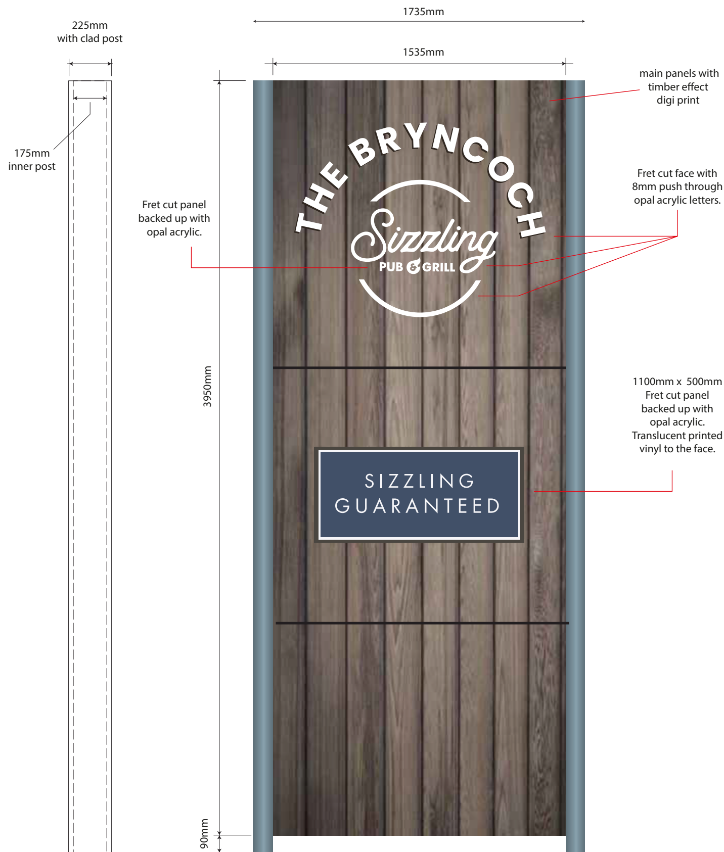
ITEM 4. (1 off) Refurbish double sided totem with new panels. Illumination provided by internal LED's. Posts painted by Main Contractor
