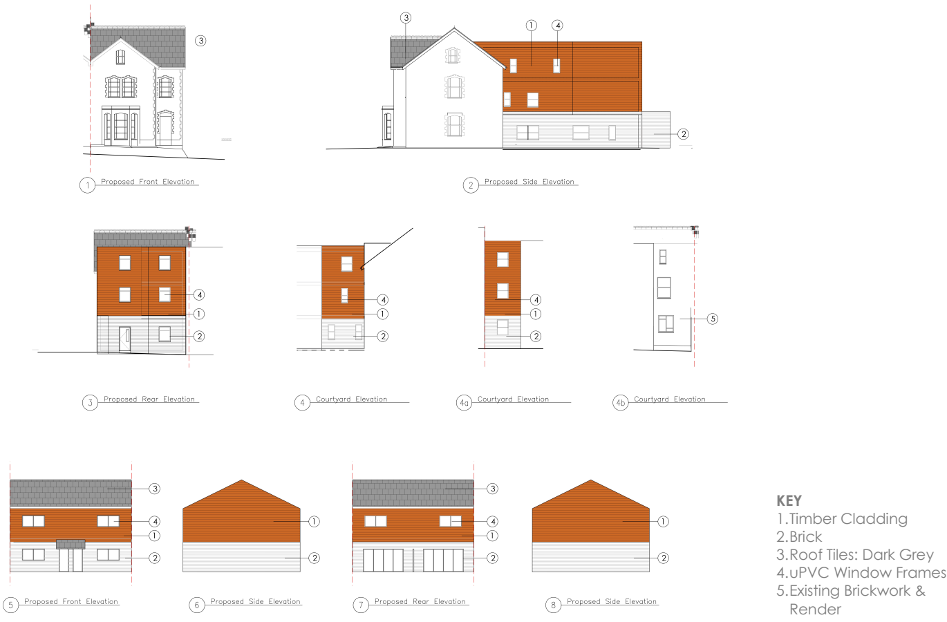
Figure 2 Elevations with External Materials
