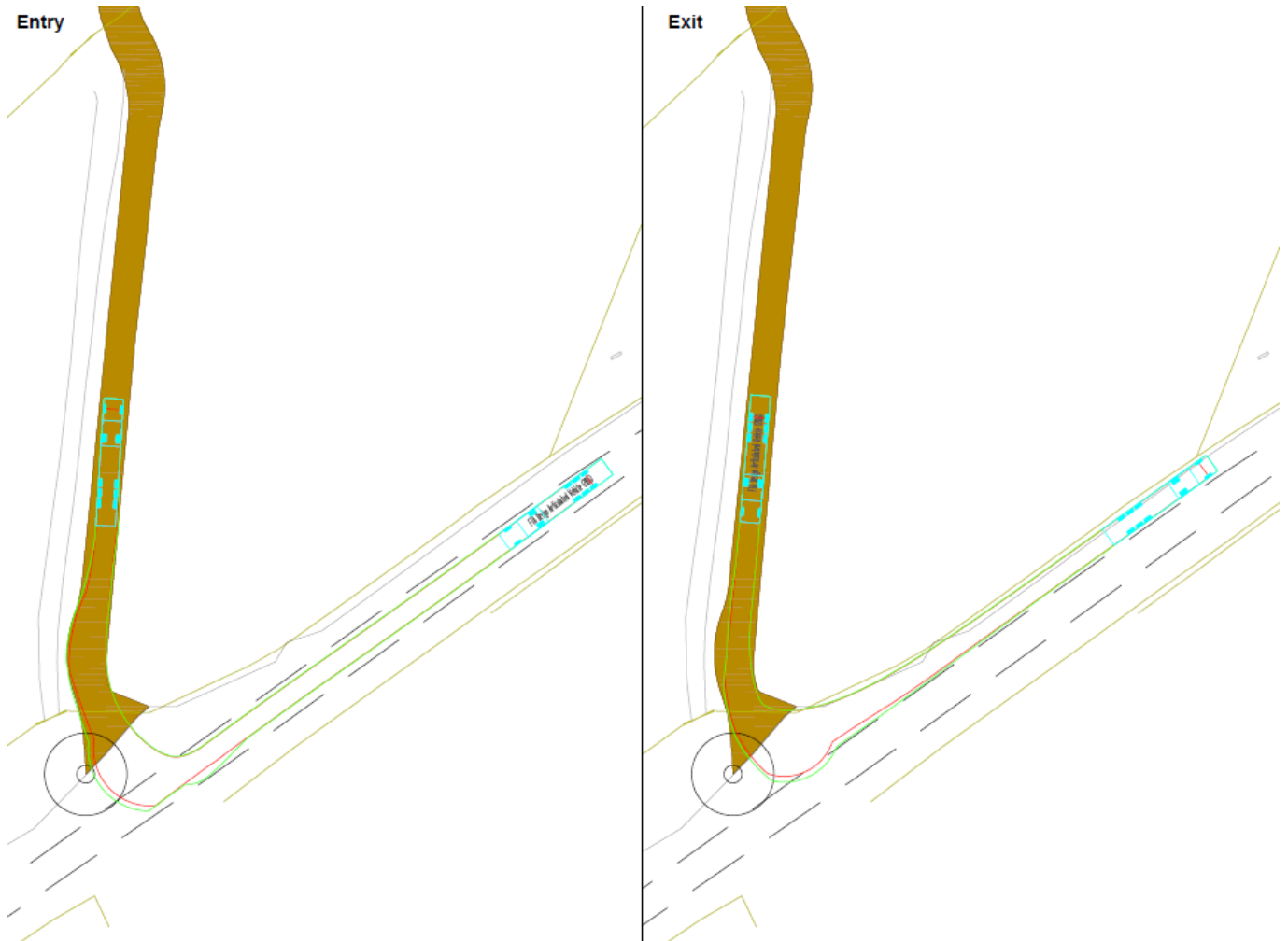
Figure 4.3: A4061 Access Swept Path Analysis
