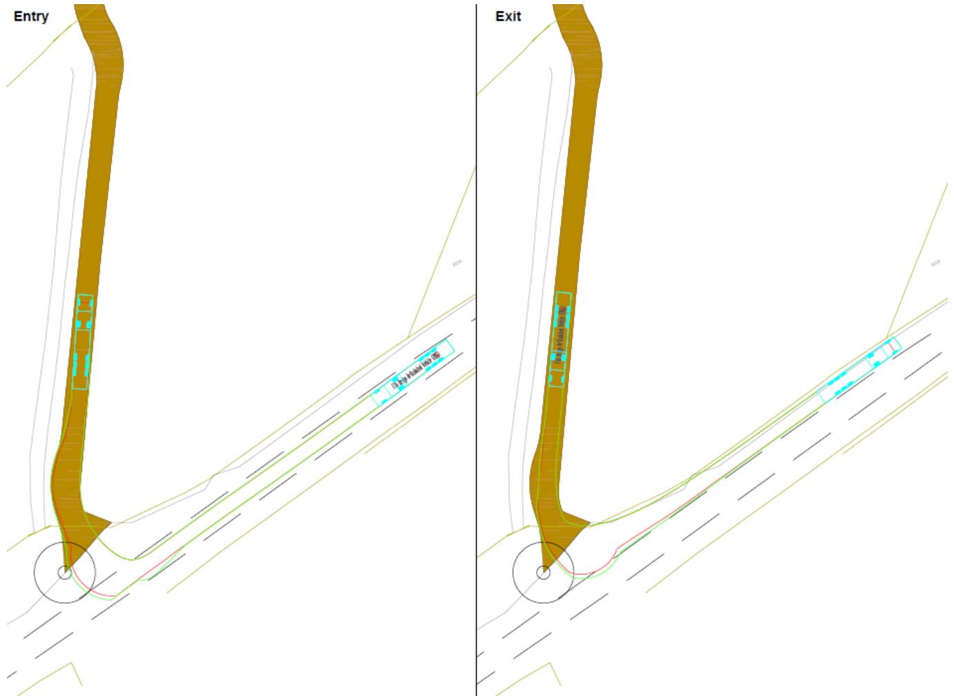
Figure 4.3: A4061 Access Swept Path Analysis
