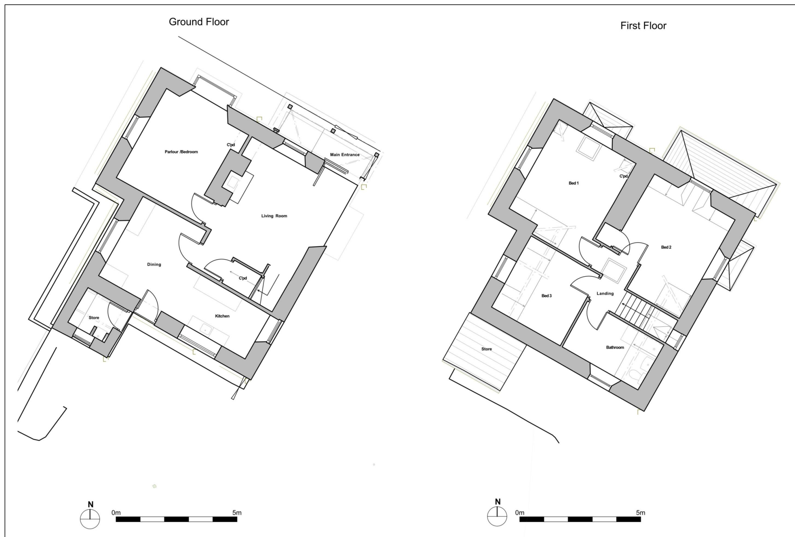
Figure 19: Plan of the ground floor and first floor of Pond Cottage. Based on drawings produced by Hiraeth for Andrew Scott Ltd (drawings 01031/S2/P2 and 01032/S2/P2) with adaptations and annotations by DAT-AS.
