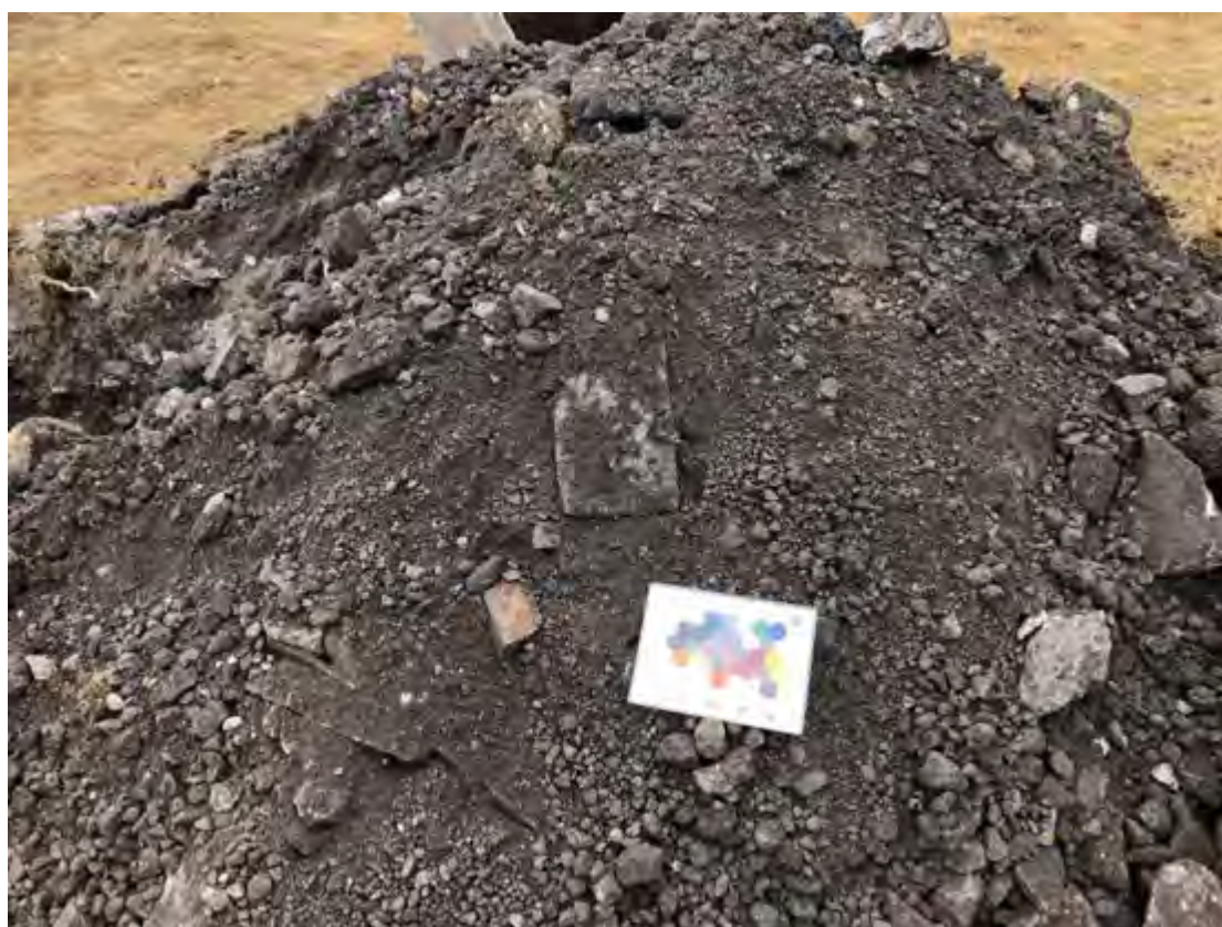
Photograph 24: Encountered ground conditions within trial pit, TP217.
