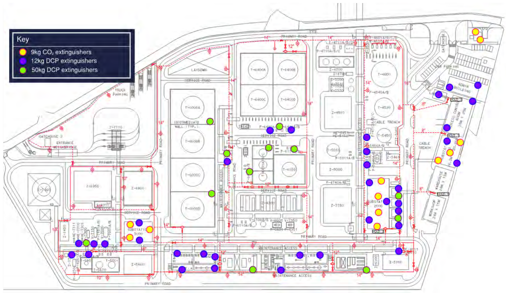
Figure 13: Project Dragon Proposed Extinguisher Layout (Source: LanzaTech Drawing)
