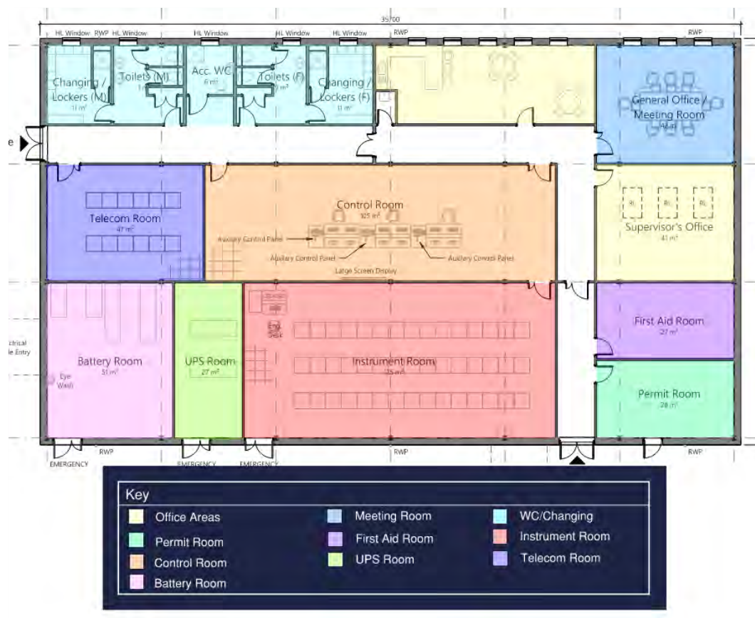
Figure 18: Process Control Room - Ground Floor (Source: Inspire Drawing)
