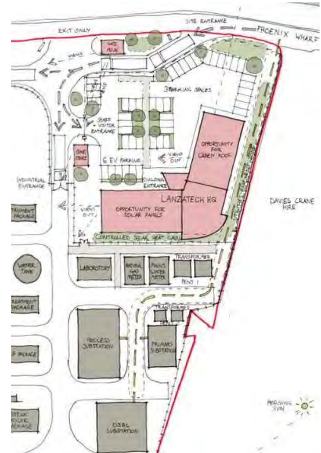
Figure 67 – Early-stage development of building arrangement, site access and building form. It was later decided to move the process control building out of the administration area into the industrial process area of the PDZ. This assists in communication and control of security for the facility.
