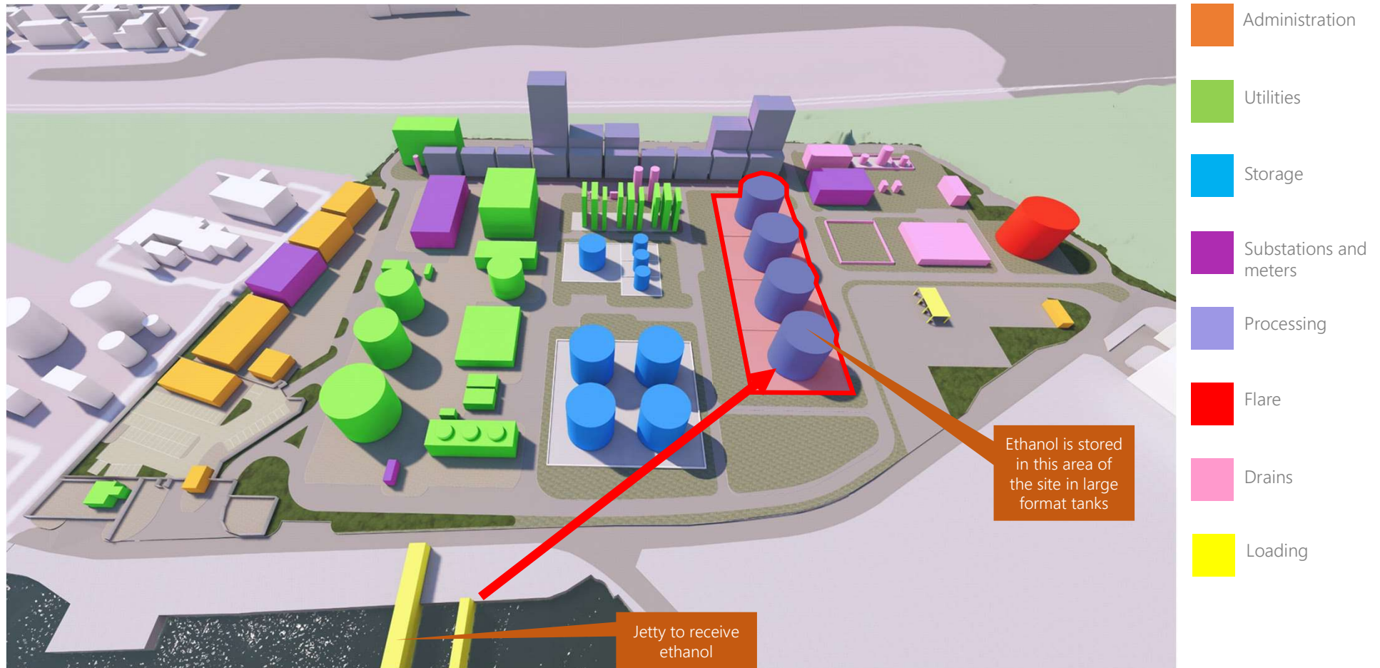
Figure 59 – Receipt of Ethanol feedstock and on-site storage. Feedstocks and products from the plant will pass to the jetty via below ground pipeworks.
