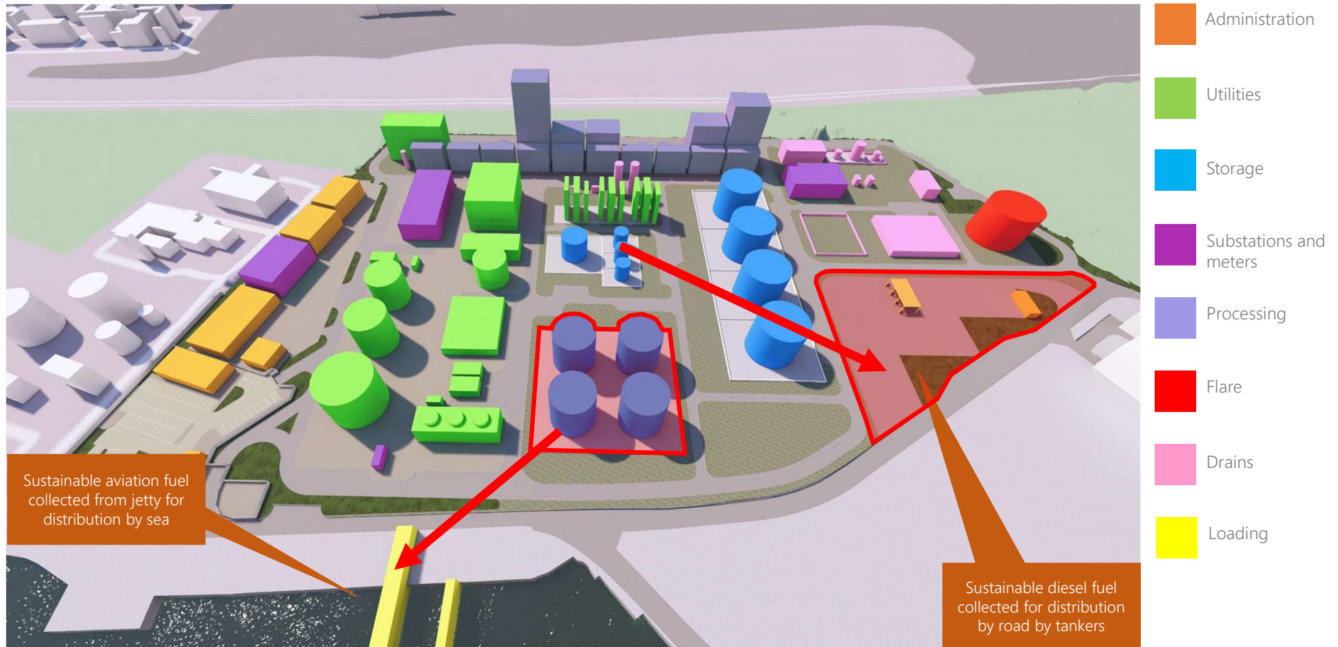
Figure 64 – Distribution of finished products. Products will be moved around the site via pipe runs that are not shown in this diagram for clarity. For details of pipe runs refer to the architectural drawings.
