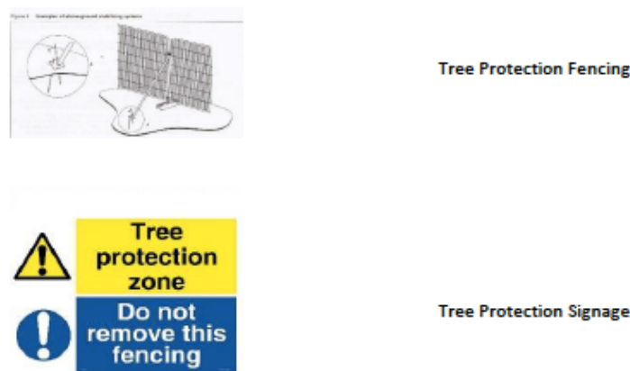
Figure 3: Tree Protection Fencing and Signage examples
