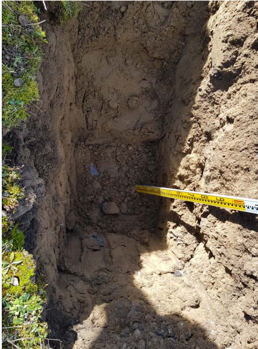
Figure 2 – Trial Pit Drained. Good illustration of the sandy substrate
