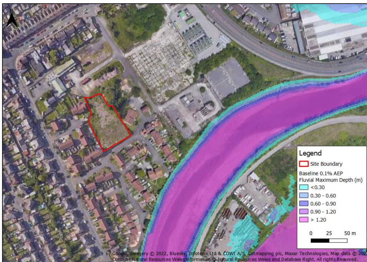
Figure 5-1 Baseline Fluvial 0.1% AEP – Fluvial
