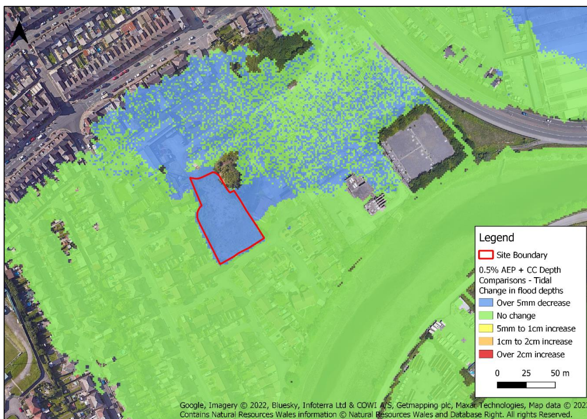
Figure 5-6 Comparison of pre- and post-development in the 0.5% AEP + Climate Change event
