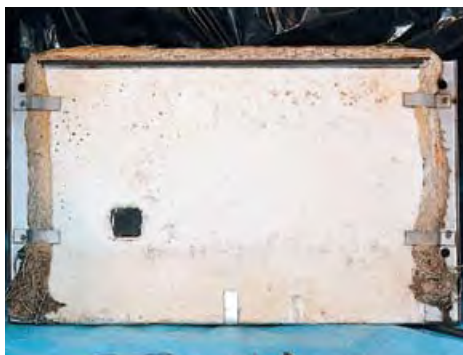
Figure 21 Asbestos rope seal and soft panelling on the burner/heat exchanger of a domestic boiler
