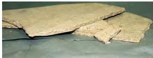
Figure 31 Asbestos cement generally contains 10–15% asbestos fibre bound in a cement matrix. Because the fibres are firmly bound in the cement matrix they will only be released if the material is subject to significant disturbance, such as drilling or sawing
