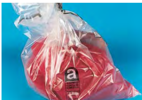
Figure 56 Asbestos waste double bagged
