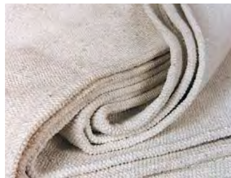
Figure 9 Asbestos fire blanket
