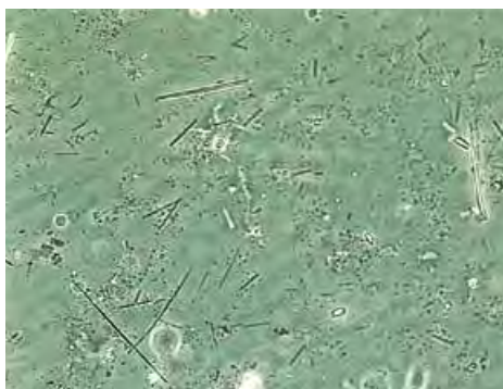
Figure 64 Microscopic (x 400 magnification) asbestos fibres (dark needle-like structures) in dust from a surface which was not cleaned properly following asbestos removal - these would not be visible to the naked eye. The dark specks and light needle-like structures are non-asbestos dust
