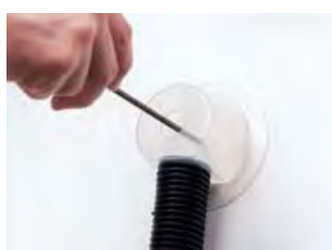
Figure 44 Using LEV during unscrewing AIB
