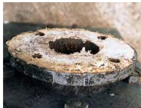
Figure 22 Debris from an asbestos gasket on a pipe flange
