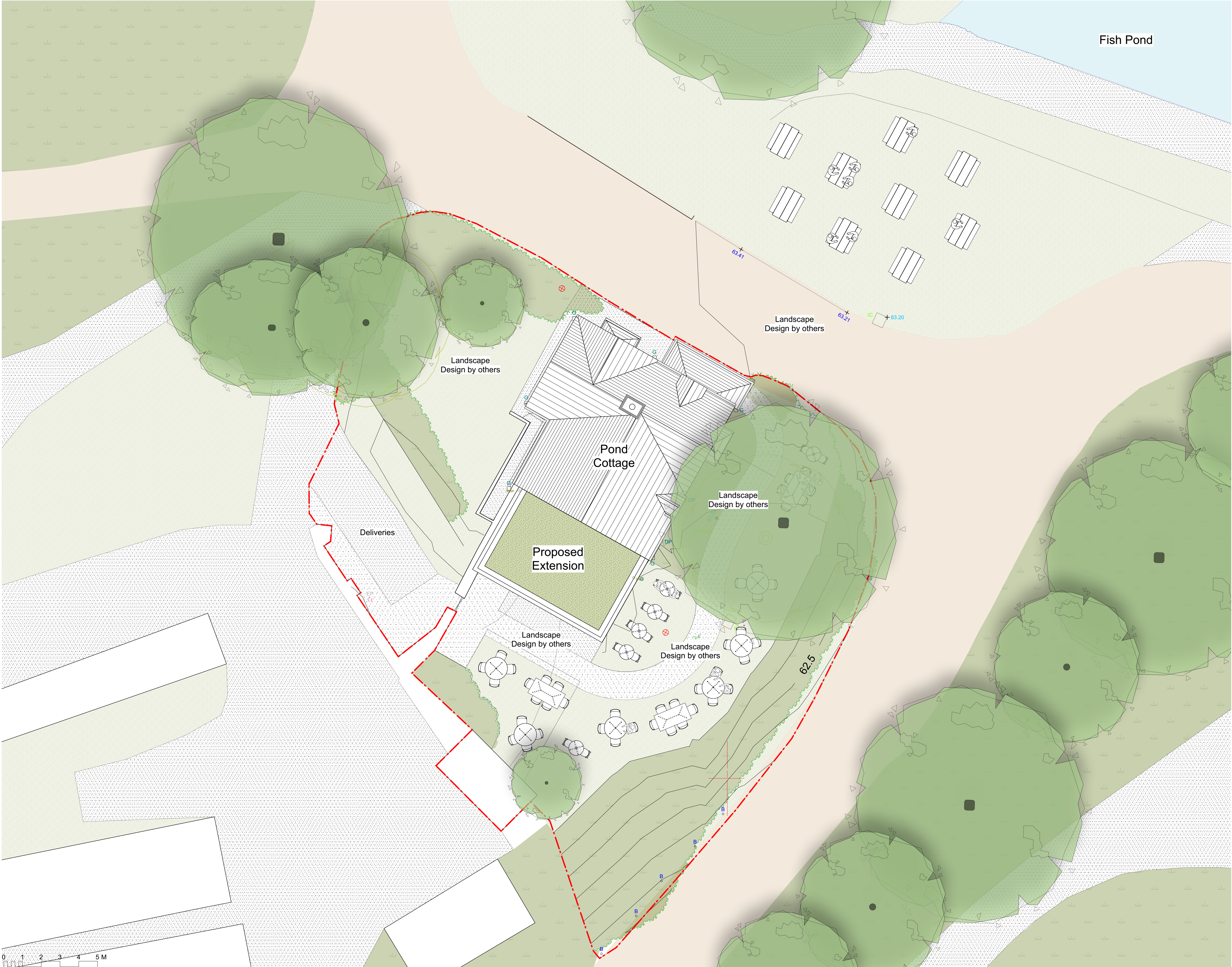
P 00201.1 PROPOSED SITE PLAN SCALE 1:100 @ A1, 1:200 @ A3
