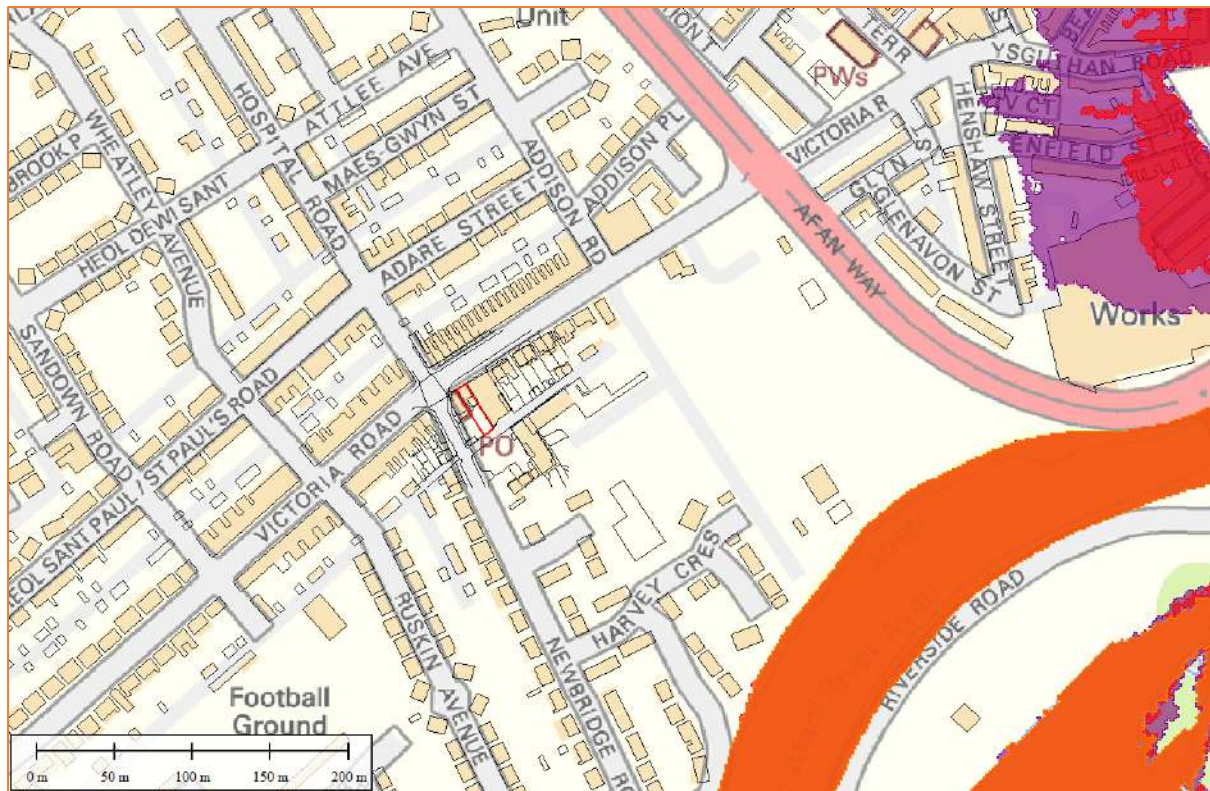
Figure 8: Modelled 1:100 year (orange), 1:100 year + CC (red) and 1:1000 year (purple) fluvial flood extents (Source: NRW, OS Mapping)
