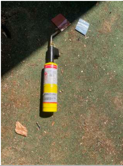
Gas blow torch used to aid in the adherence of the PAG SAGR.
