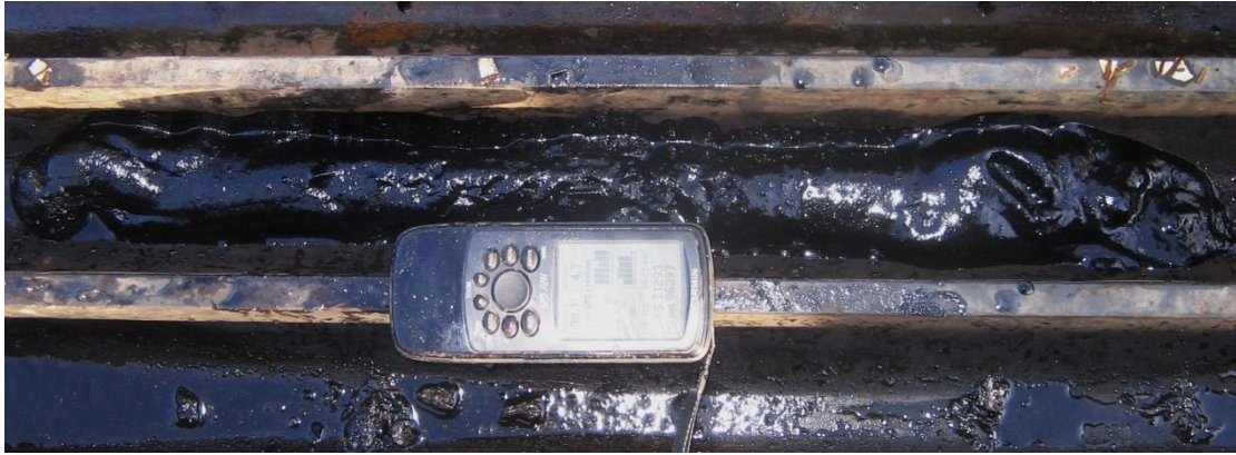
Photograph 1: Sample of sludge prior to dredging works
