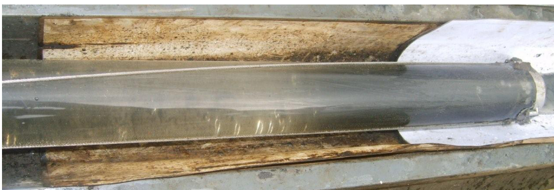
Photographs 5: Shows the sampling probe discharging a sample
