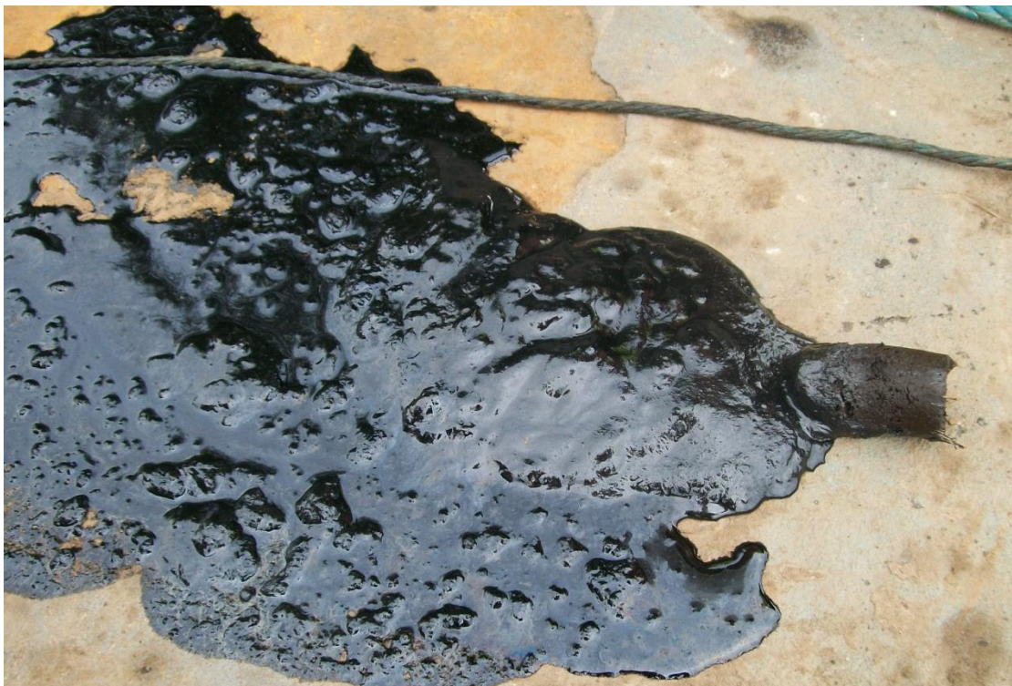
Photograph 3: Sample of sludge on a flat surface with plug of underlying natural material
