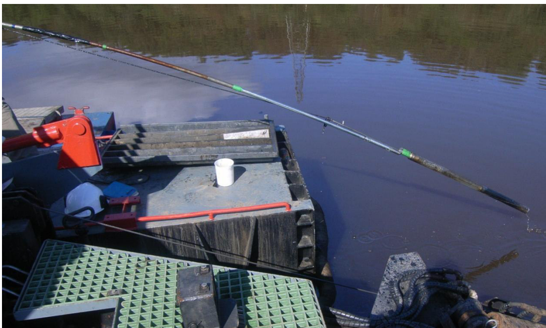
Photograph 6: Sampling probe with extension poles retrieving a sample
