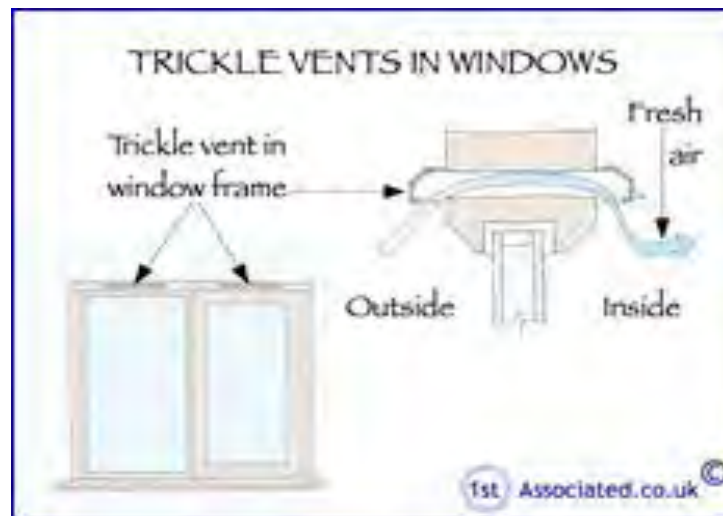
Figure 1 : Trickle Vents to Window Frames
