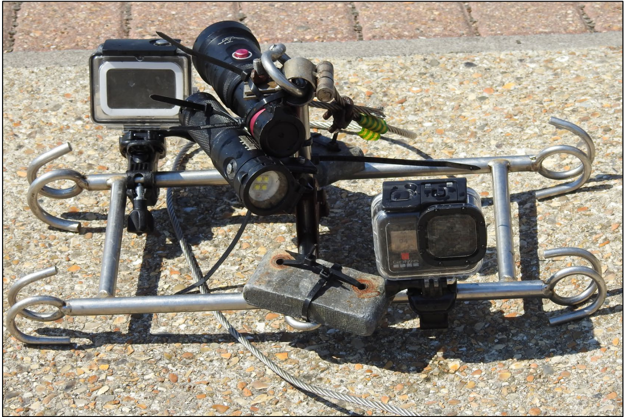
Figure 3. The Drop-down video (DDV) system used during the subtidal survey
