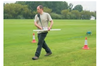
GEM-2 Multi-frequency Exploration depth up to 10m
