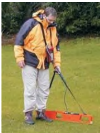
EM-38 Single frequency Exploration depth ~1.5m
