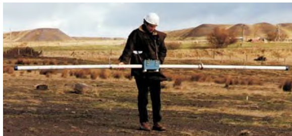
EM-31 Single frequency Exploration depth ~3 to 5m
