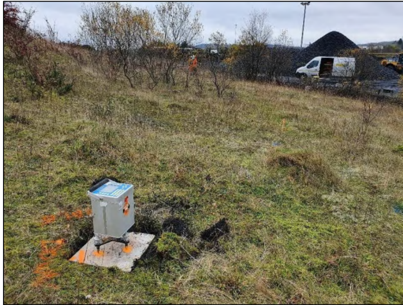
Plate 5: Microgravity survey with Scintrex CG-5 instrument in Zone 1
