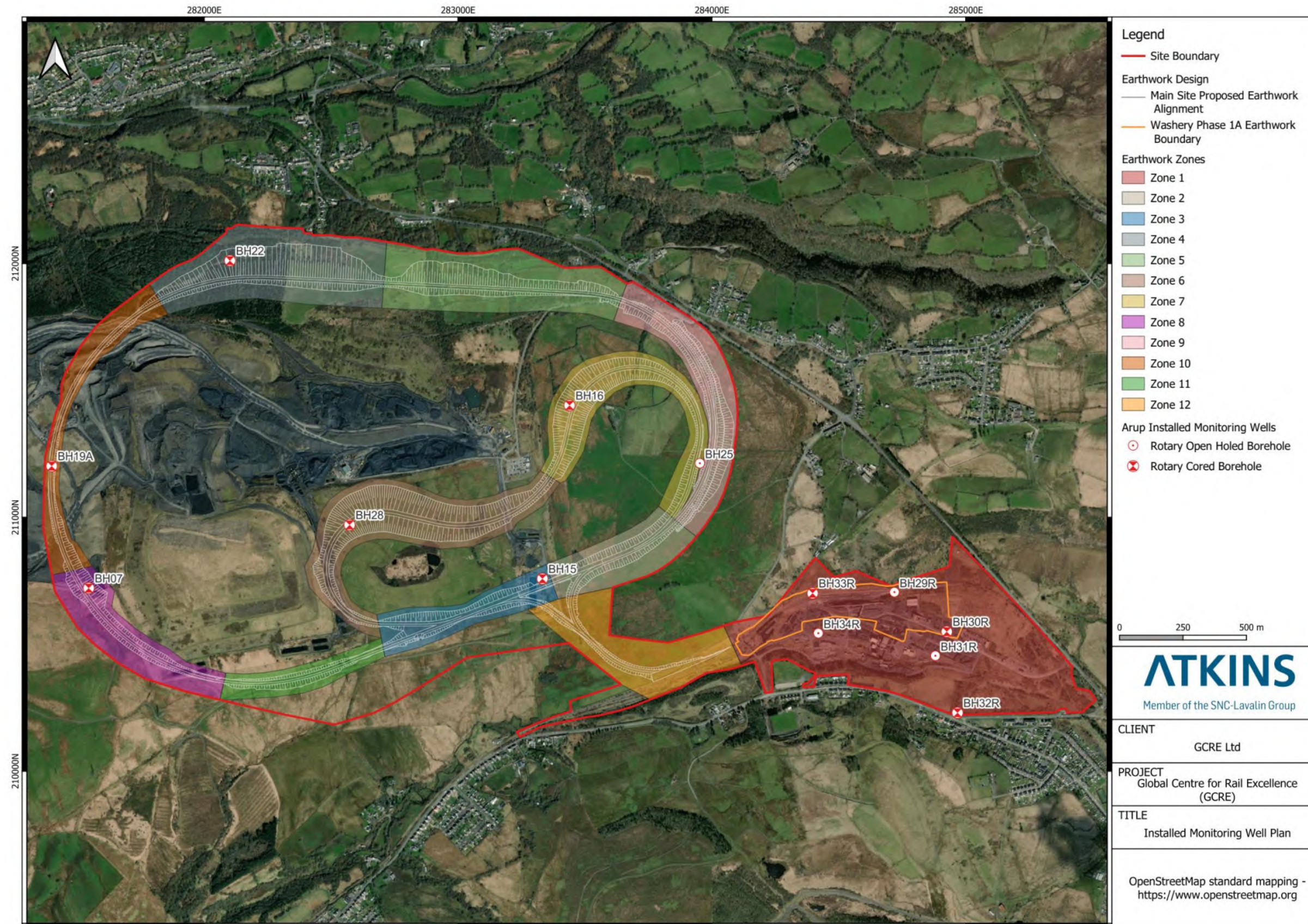
Figure 7-1: Installed Monitoring Well Plan.
