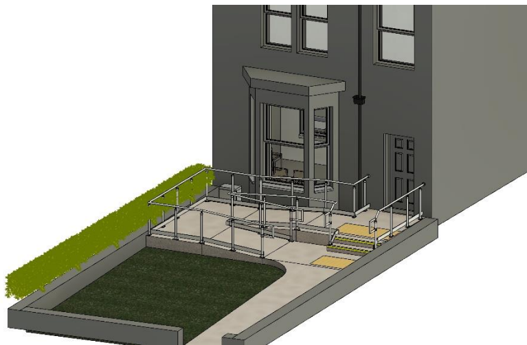
Figure 2 - Ramp to Front (Right View)
