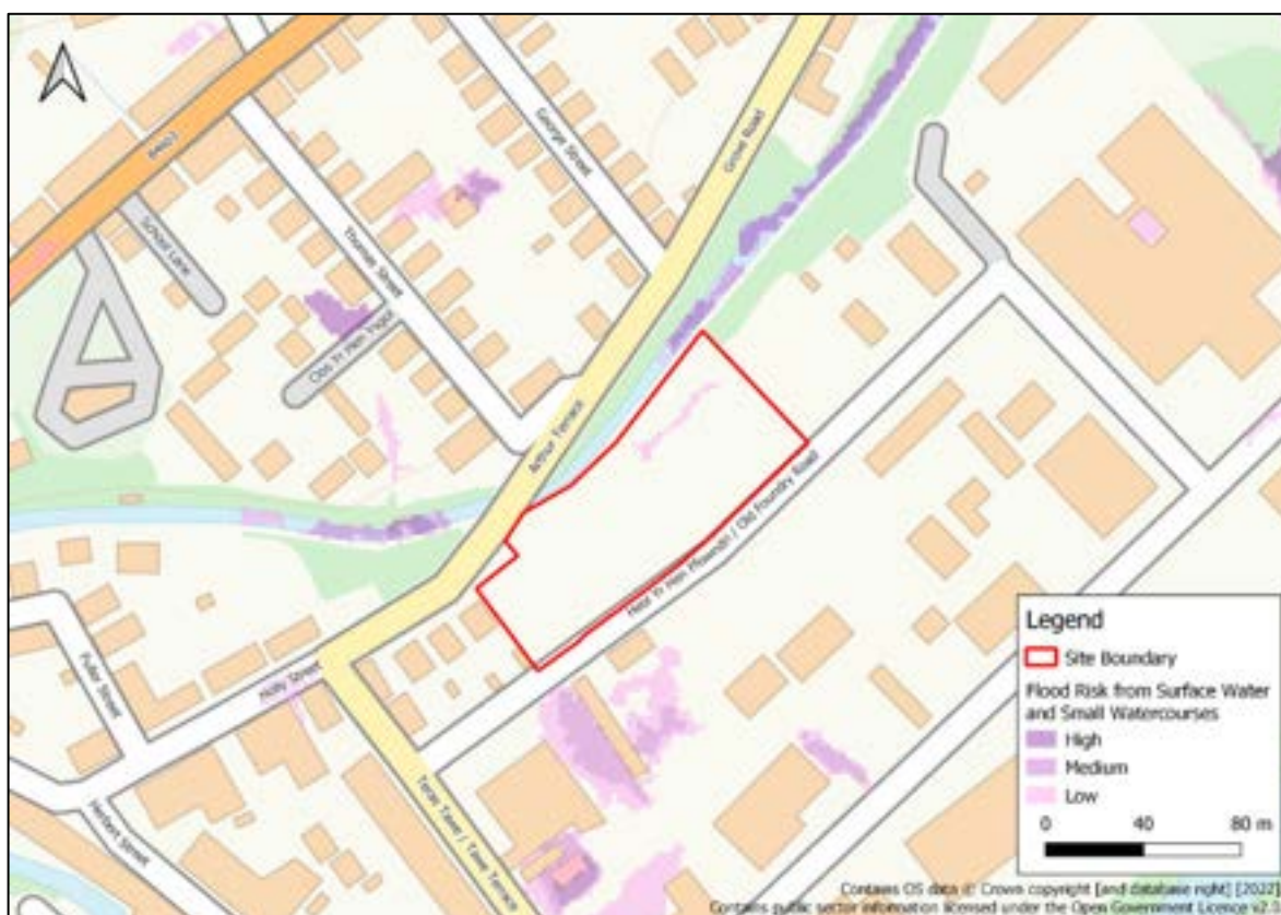
Figure 4-2 FRAW map – Risk of flooding from Surface Water and Small Watercourses
