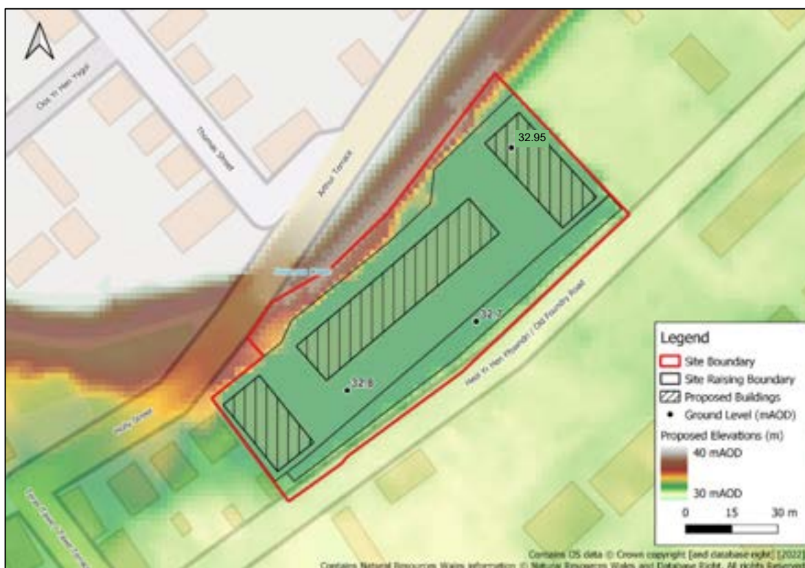
Figure 5-3: Post-development site layout and levels
