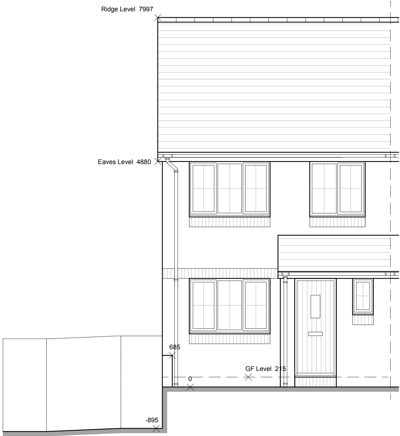
EXISTING FRONT SECTION A-A 1:50
