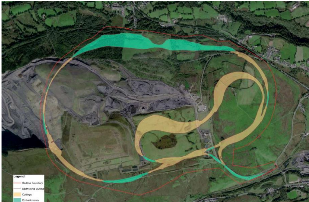
Figure 1 – Earthworks area showing cuttings and embankments
