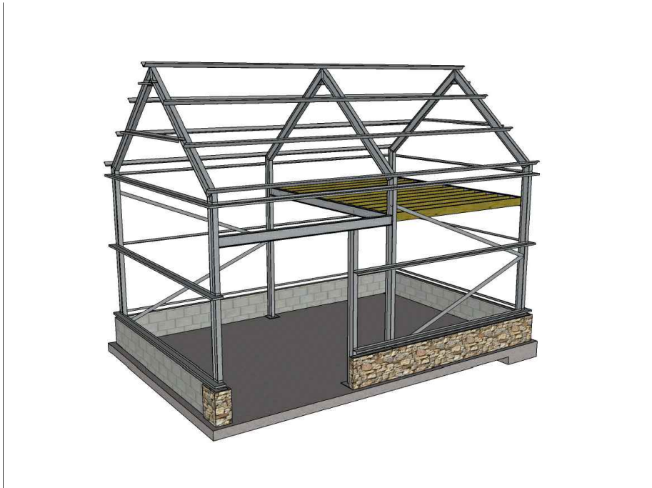
Pic.12 Z Section galvanised purlins as cladding rails to walls and roof
