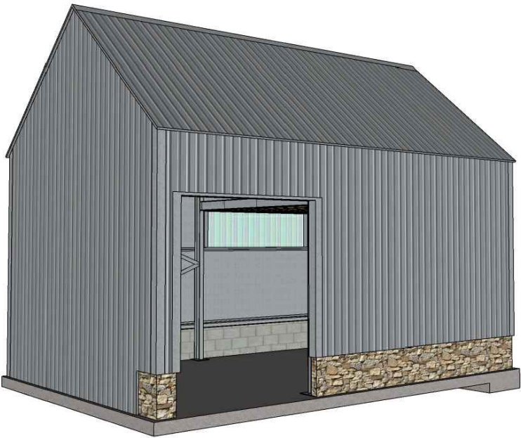
Pic. 17 Front & Side Elevation (North West). Vehicle Entrance Opening dimension appx 2800 wide x 3300 height) 'Barn Door' style on existing although replacement likely to be proposed as roller shutter
