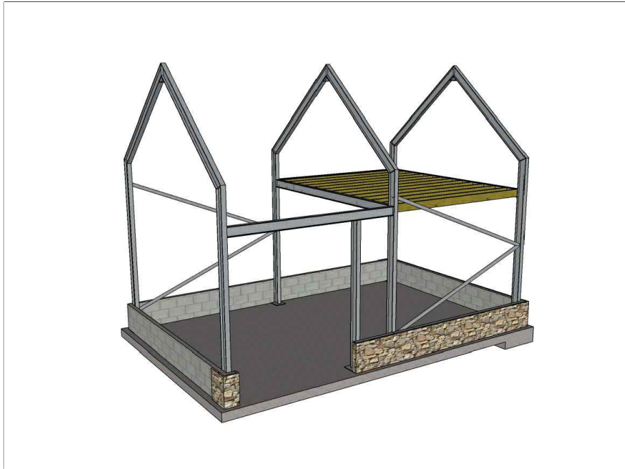
Pic.11 Tanalised timber joists spanning between structural suspended floor members to provide storage accommodation to domestic floor standard capacity (1.5kN/m2). P5 Grade 18mm T&G flooring as deck. Soffit left exposed.
