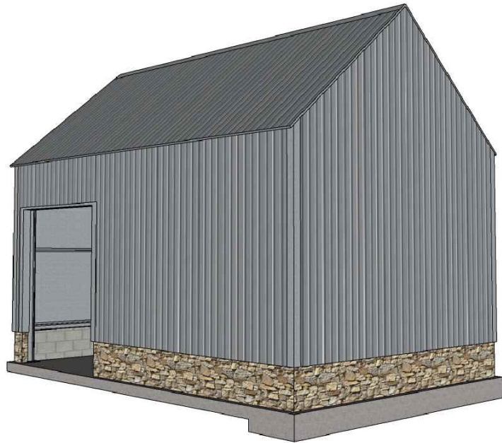
Pic. 14 Front & Side Aspect Elevation (South West) Galvanised 32/1000 metal profile sheet cladding to walls and roof Natural stone cladding to height of approximately 650 mm
