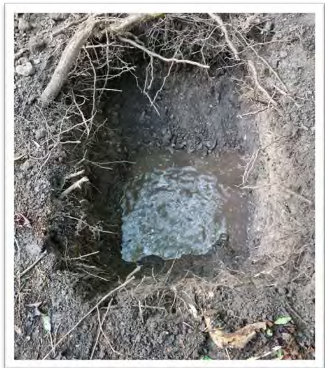
Figures 3: Trial Pit Towards the End of Testing
