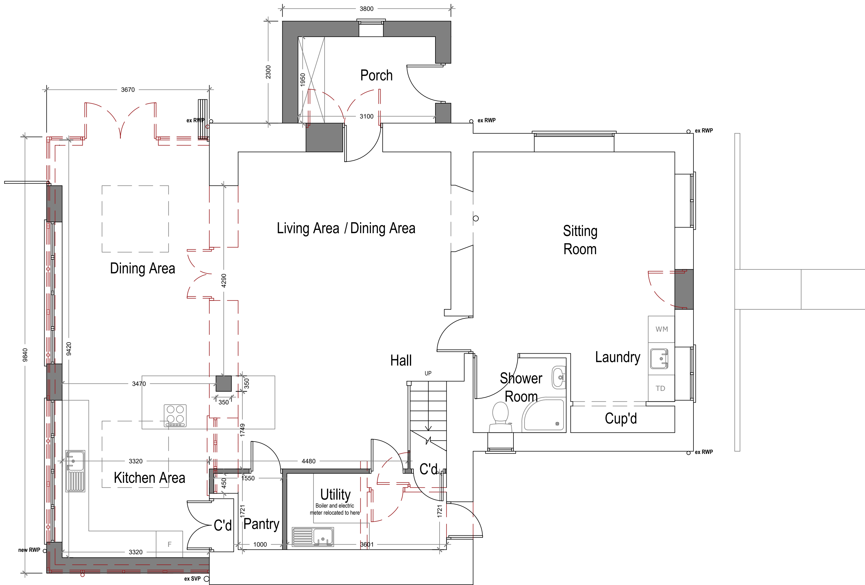
Proposed Ground Floor Plan Scale 1:50 Area ca. 118.78 m² Additional Area: 2.30 m²
