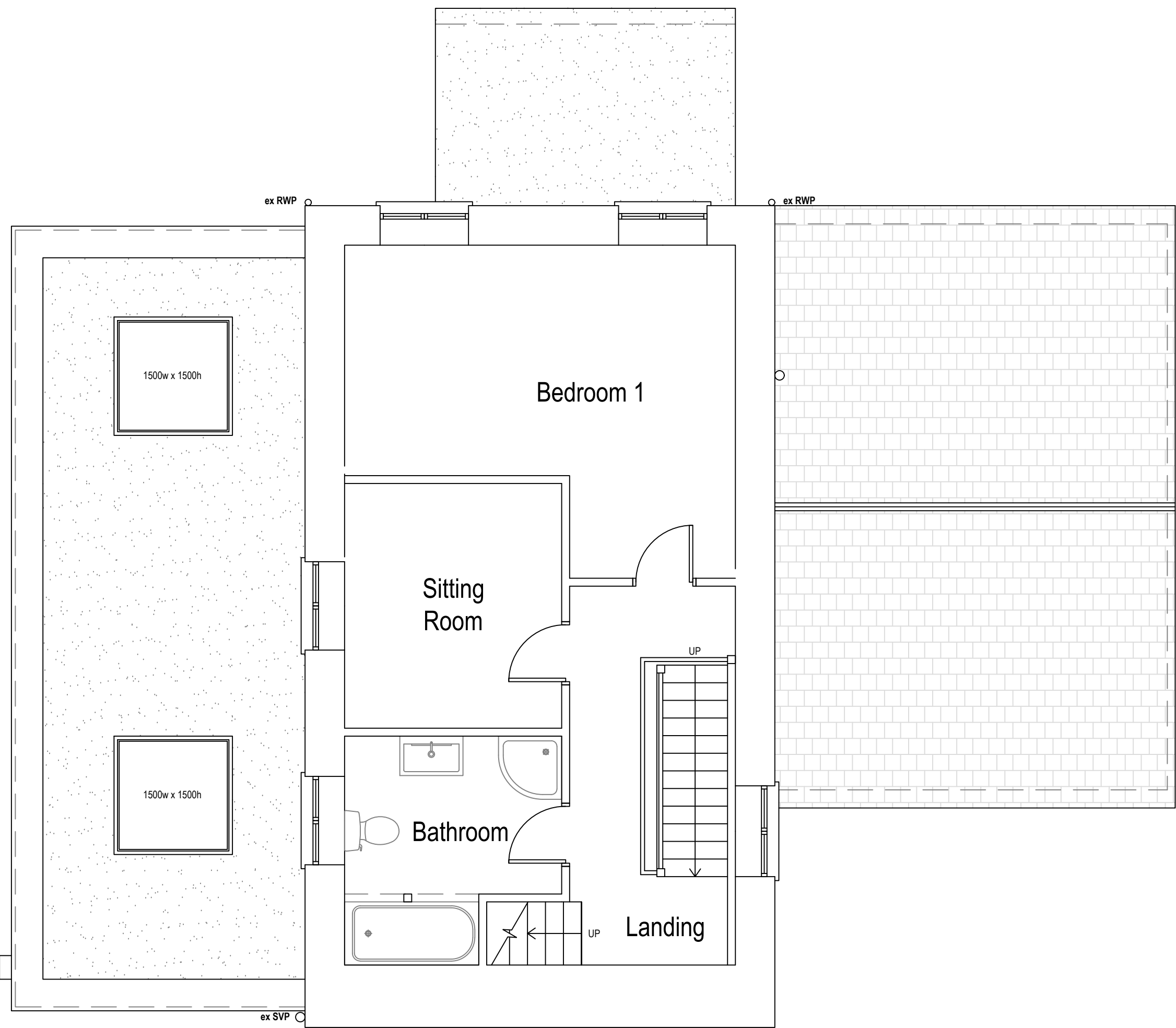
Proposed First Floor Plan Scale 1:50 Area ca. 45.14 m²
