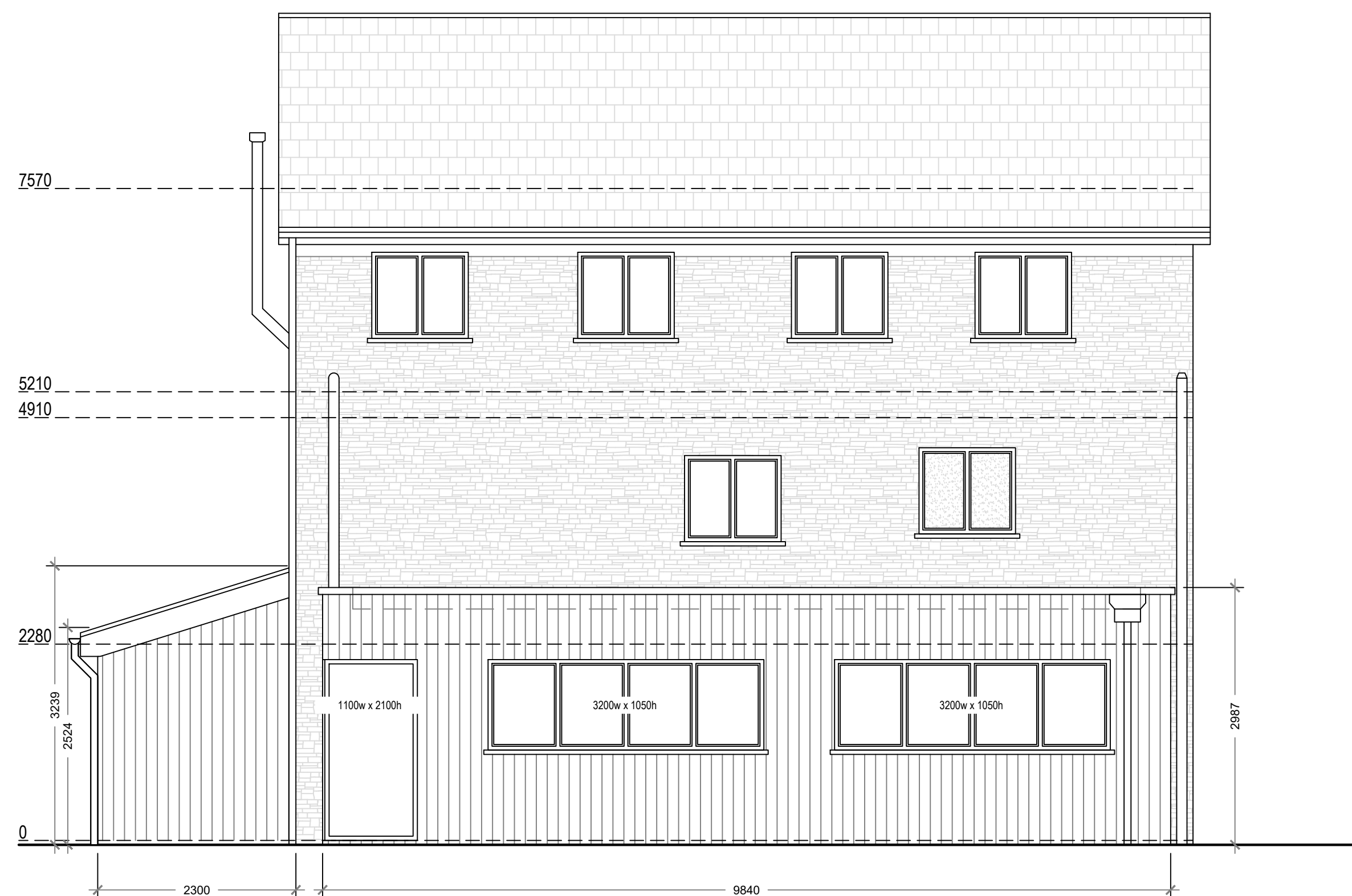
Proposed Southeast Elevation Scale 1:50
