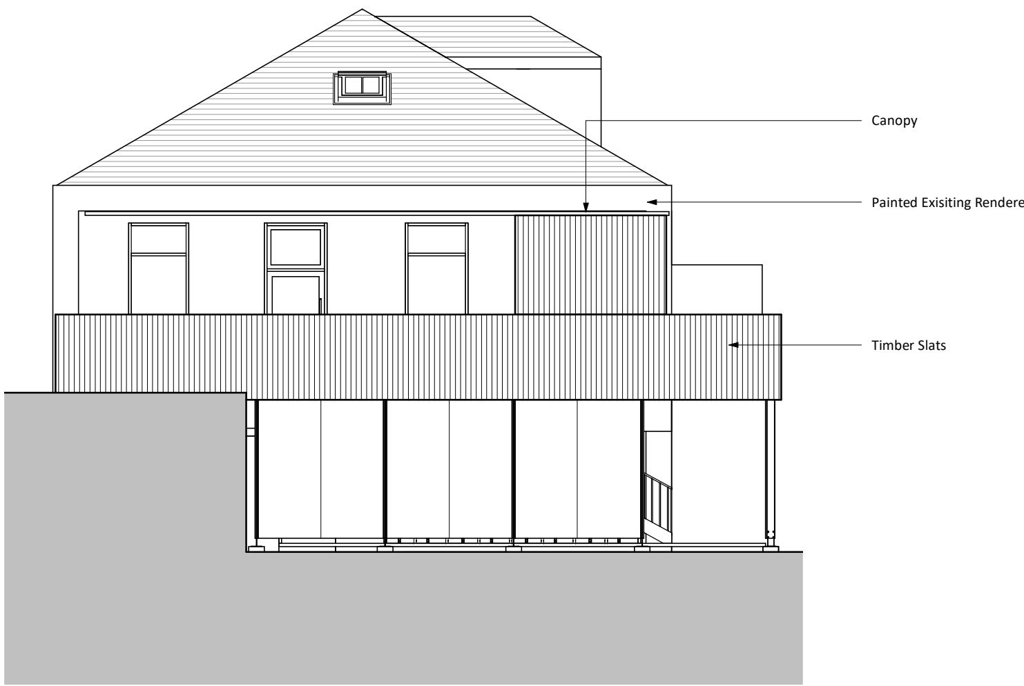
Proposed East Elevation 1 : 100
