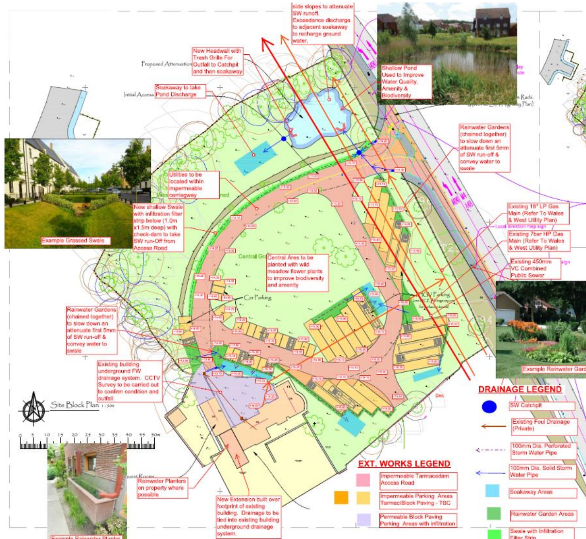
Figure 24 – proposed drainage scheme at Tyn-y-Caeau
