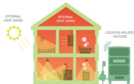
Figure 18 – Contributing Factors, Overheating
