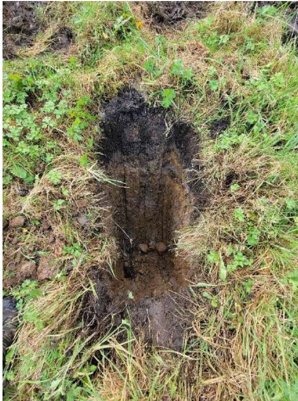
Picture 1 – Test Pit 1 Soil Strata. No water at base
