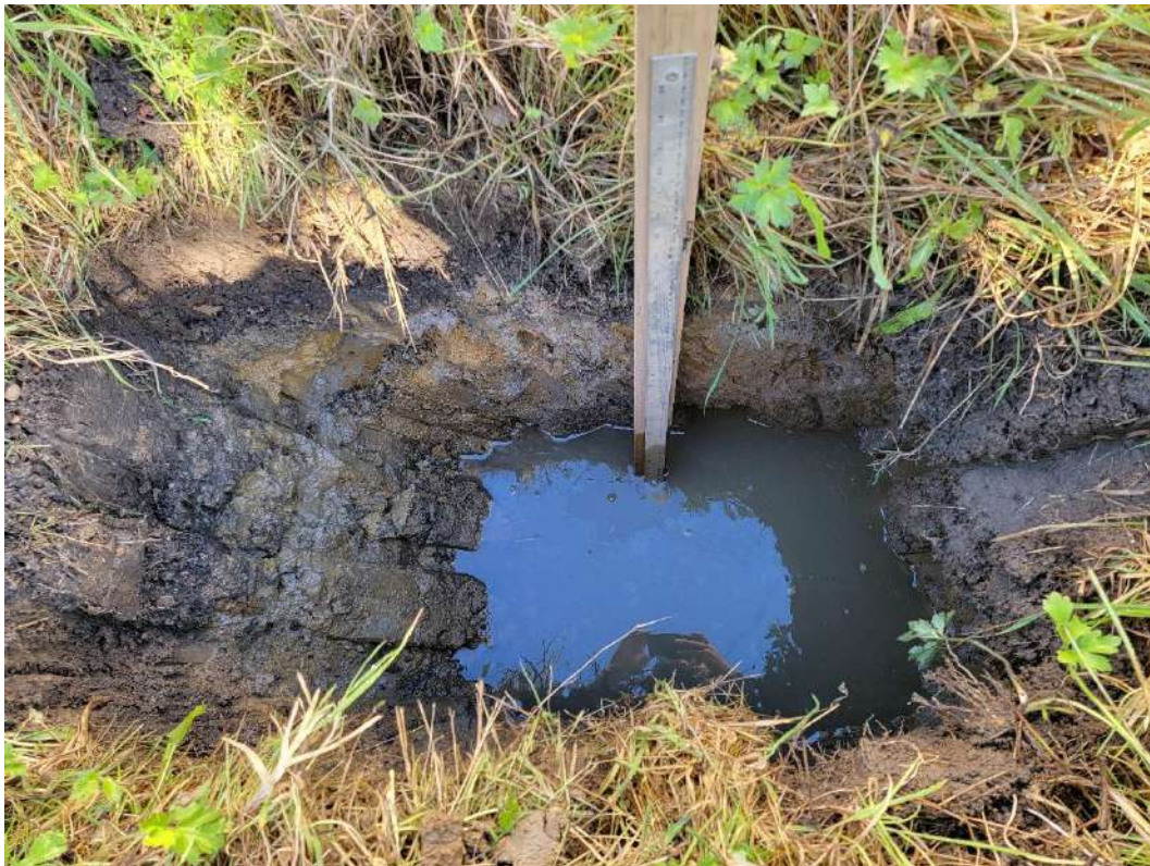
Picture 6 – Condition of Test pit 1 the morning of testing following heavy rain.
