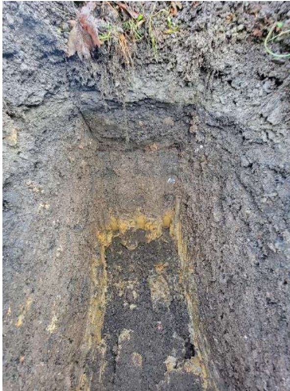
Picture 5 – Test Pit 2 Ground Strata's
