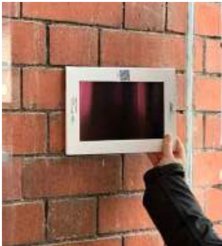
Varying the viewing angle of the dichroic stainless steel reveals different colours, as shown against the Arts Centre brick.
