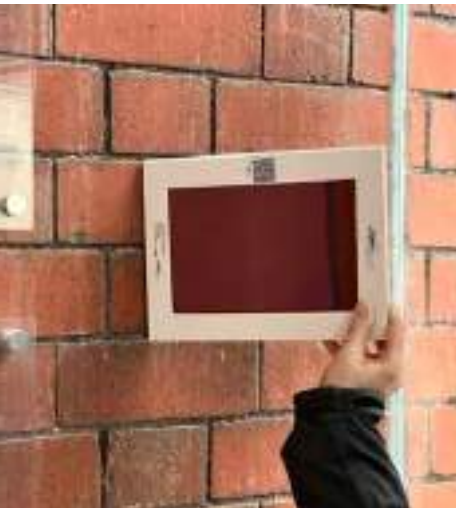
Varying the viewing angle of the dichroic stainless steel reveals different colours, as shown against the Arts Centre brick.
