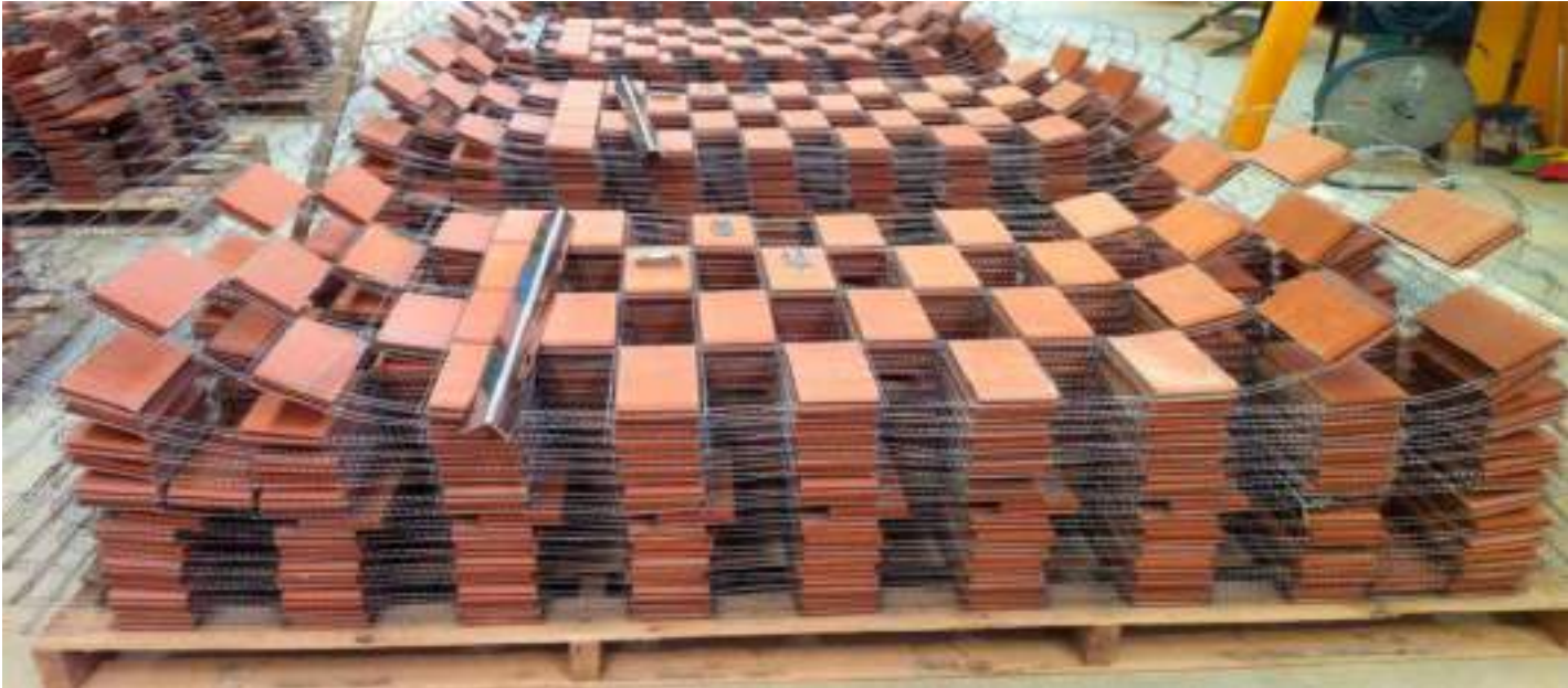
Flexbrick units within wire mesh system.
