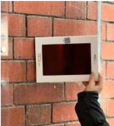
Varying the viewing angle of the dichroic stainless steel reveals different colours, as shown against the Arts Centre brick.
