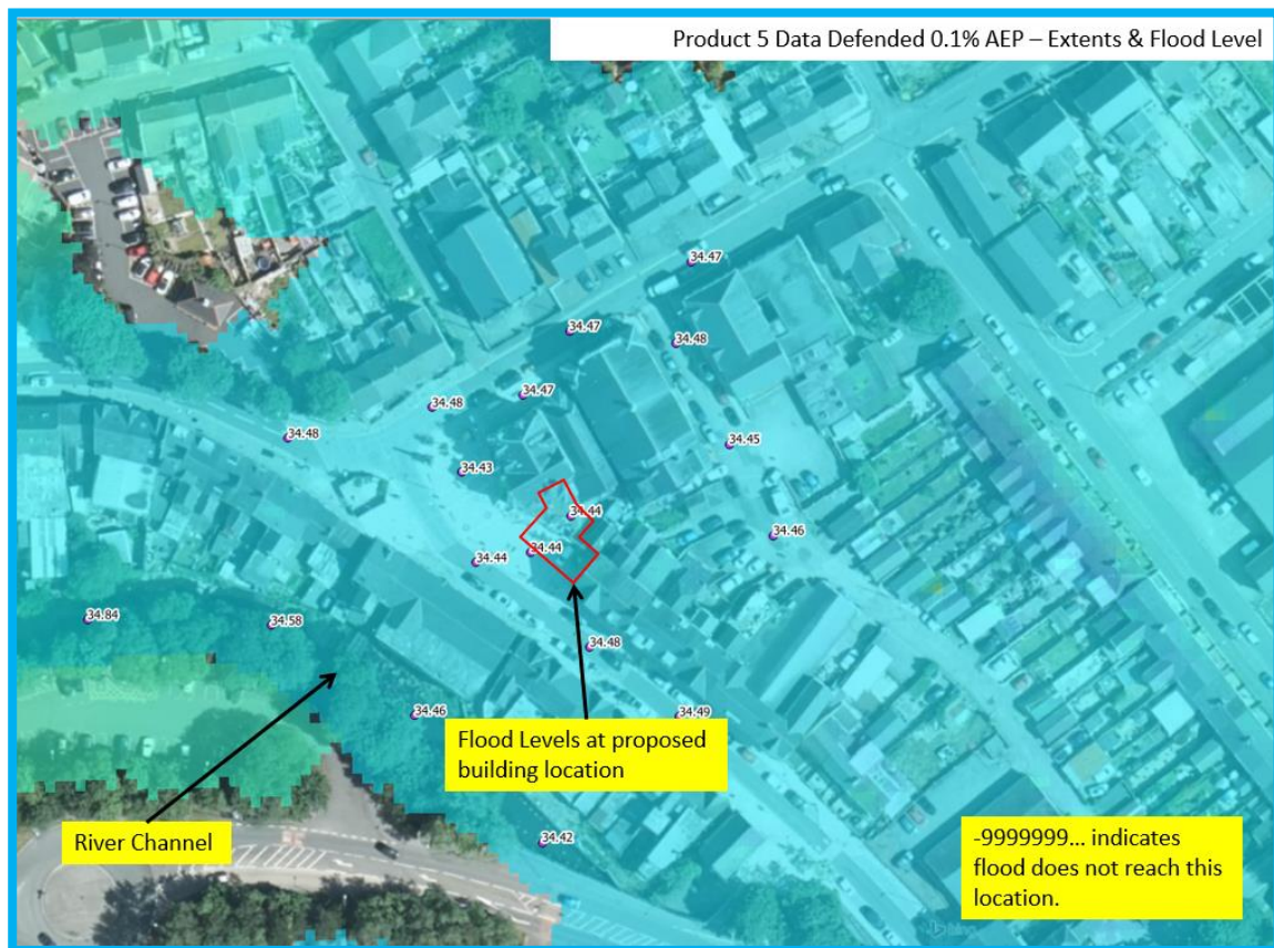
Fig 11 0.1% AEP event shows 1.4m depth of flooding at the site
