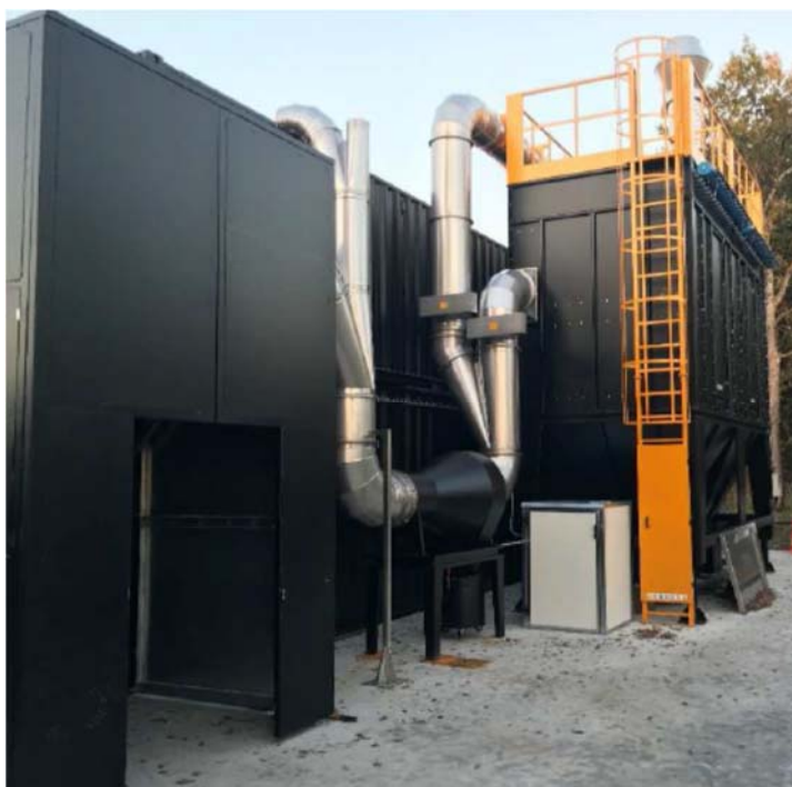
Filter housing with ducting, fan, spark separator, pre-coating dosing station and stack (Example La Roche / France)
