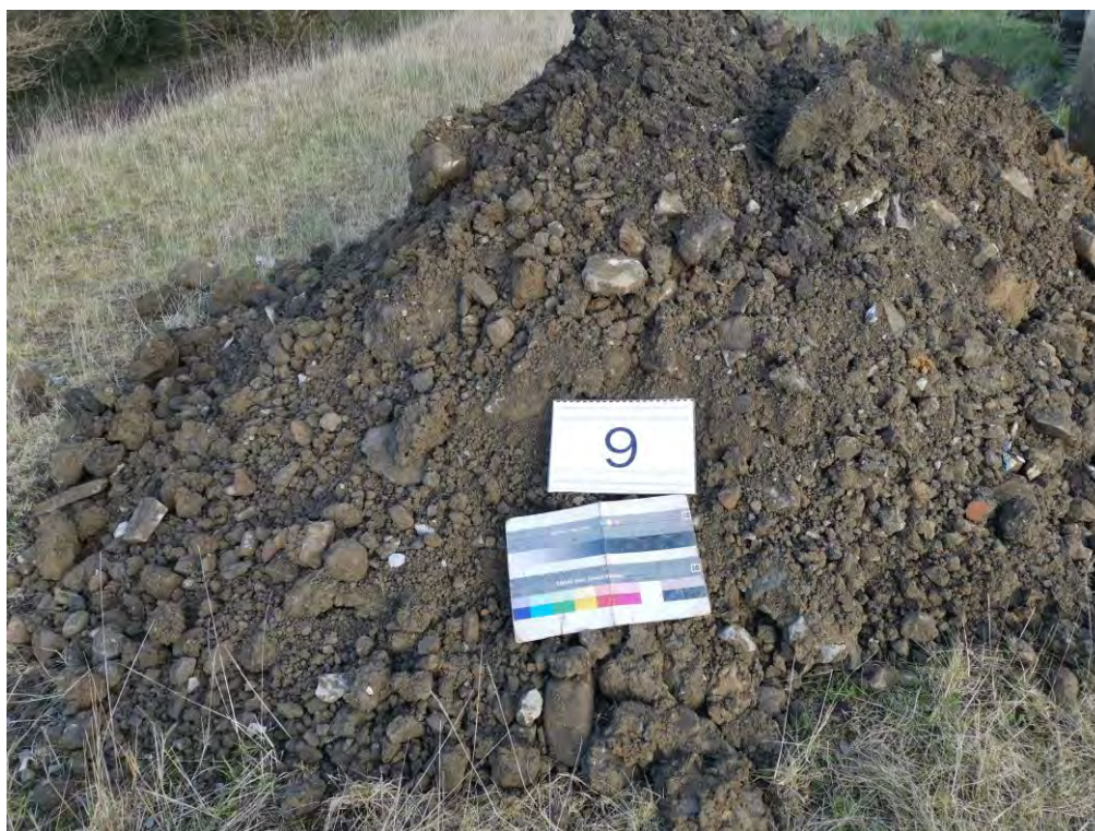
Plate 9: Fill A material arisings excavated from TP09.
